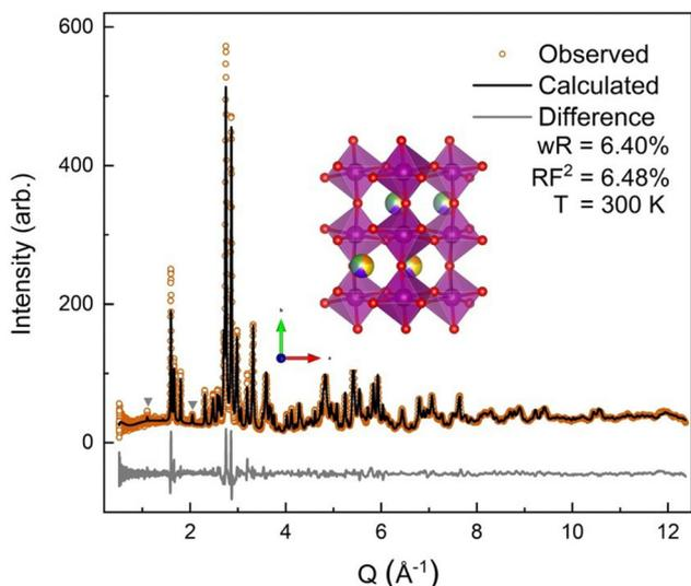
Fig. 4 Room temperature neutron powder diffraction data. The orange circles denote the observed neutron diffraction intensities, the black line is the calculated fit from GSAS-II with a  $wR$  of 6.40% and a main phase  $RF^2$  of 6.48%. The gray triangles denote YMnO<sub>3</sub> impurity peaks. The light gray line is the difference, (data-fit) shifted down for visibility.
