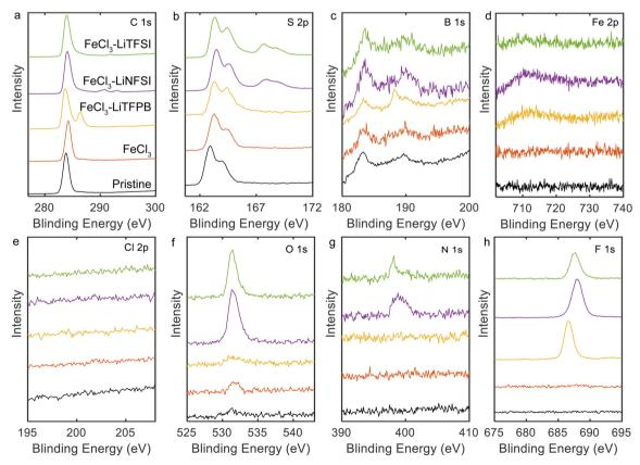
Fig. 2 XPS spectra of doped PQT thin films: (a) C 1s, (b) S 2p, (c) B 1s, (d) Fe 2p, (e) Cl 2p, (f) O 1s, (g) N 1s, and (h) F 1s regions.
