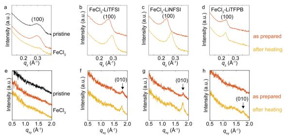
Fig. 4 XRD measurements of the doped PQT thin films. Intensities for the (a)-(d) out-of-plane and (e)-(h) in-plane directions. Orange plots were obtained from thin films after treatment with FeCl<sub>3</sub> or combinations of FeCl<sub>3</sub> and additional salts. Yellow plots were obtained after heating the treated samples at 125 °C under air.
