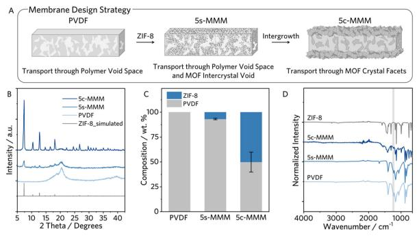
Fig. 2 (A) Membrane design strategy. (B) PXRD, (C) estimated composition, and (D) FTIR of PVDF, 5s-MMM, and 5c-MMM. Composition is determined by <sup>1</sup>H NMR digestion experiment.
