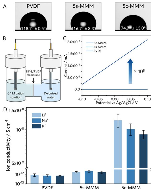
Fig. 4 (A) Water contact angle measurements of PVDF, 5s-MMM and 5c-MMM surfaces. (B) Schematic of H-cell for measuring ion conductivity. (C) The current-voltage curve of PVDF, 5s-MMM, and 5c-MMM measured in an H-cell with 0.1 M Li ion concentration gradient across the MMM. (D) Ion conductivity extrapolated from LSV measurements and normalized to aqueous ion mobility.
