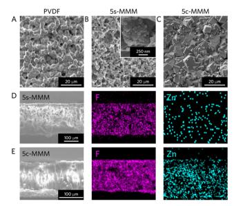
Fig. 3 Surface SEM image of (A) PVDF, (B) 5s-MMM, and (C) 5c-MMM. Inset in (B): FE-SEM detailing nanocrystalline ZIF-8. Cross-sectional SEM image of (D) 5s-MMM and (E) 5c-MMM with high resolution F and Zn mapping, respectively.
