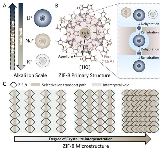
**Fig. 1** (A) Relative scale of ionic and hydrated alkali metal cations. (B) [110] facet of the ZIF-8 and schematic of ion transport. (C) Strategies to mitigate transport through intercrystal void by targeting continuous morphologies of interpenetrated ZIF-8 crystallites.
