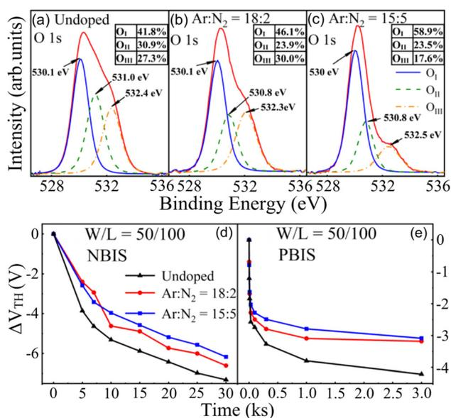
Fig. 15 Measured and deconvoluted XPS spectra of O 1s for (a) undoped, (b) Ar/N<sub>2</sub> = 18:2, and (c) Ar/N<sub>2</sub> = 15:5.  $V_{TH}$  degradation amount of TFTs with different N-doping conditions under (d) NBIS and (e) PBIS. Reproduced with permission.<sup>131</sup> Copyright 2024, IEEE Transactions on Electron Devices.
