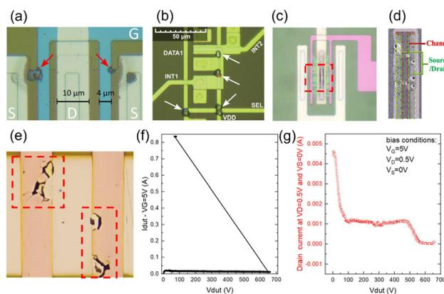
Fig. 21 (a)–(e) Surface morphology of ESD stress-induced damage on TFTs. (f) ESD-induced fluctuations in transient voltage and current and (g) DC leakage current. Reproduced with permission.<sup>167–170</sup> Copyright 2024, IEEE Journal of Display Technology, Microelectronics Reliability, M. Scholz, Microelectronics Reliability, respectively.
