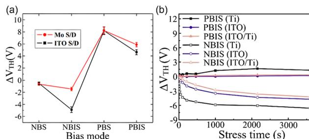
Fig. 16 (a)  $\Delta V_{TH}$  values of the IGZO TFTs using ITO and Mo electrodes under NBS, NBIS, PBS and PBIS conditions. (b)  $\Delta V_{TH}$  values of the IGZO TFTs using Ti, ITO and ITO/Ti electrodes under PBIS/NBIS conditions. Reproduced with permission.<sup>141,142</sup> Copyright 2024, Journal of Electroceramics, ECS journal of solid state science and technology.
