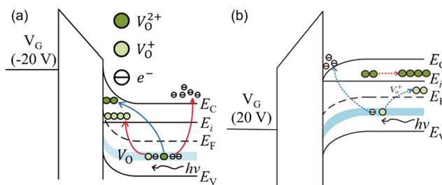
Fig. 14 Schematic energy-level diagrams of AOS TFTs under stresses of (a) NBIS and (b) PBIS, and the generation of  $V_O^+$  and  $V_O^{2+}$ . Reproduced with permission.<sup>126</sup> Copyright 2024, Chinese Physics B.
