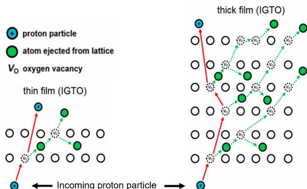
Fig. 25 Schematic diagram of the mechanism for a significant increase in the  $O_{\text{vac}}$  concentration in thicker IGTO thin films after proton irradiation based on the multiple displacement chain reaction model. Reproduced with permission.<sup>195</sup> Copyright 2024, Surface and Interfaces.
