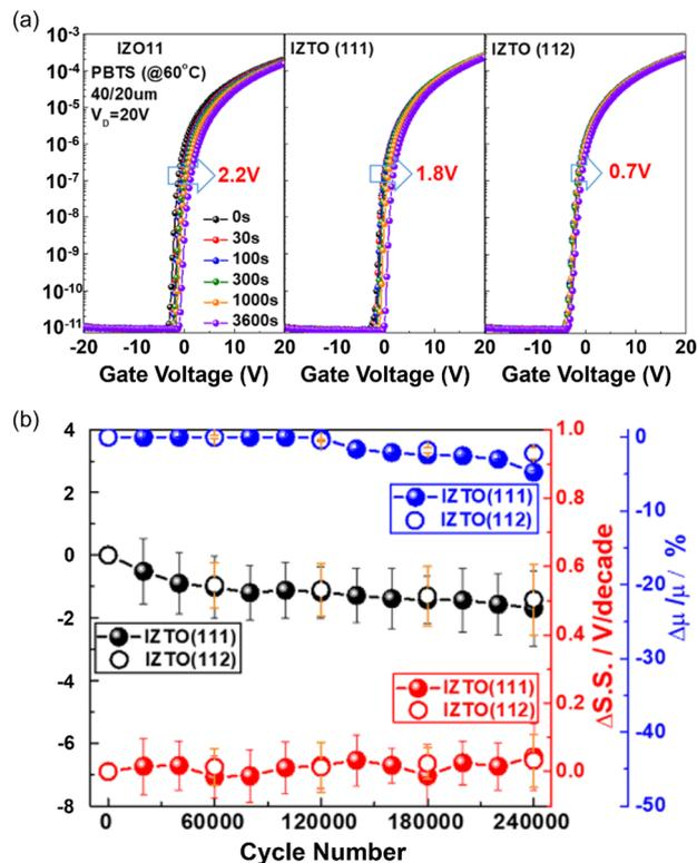
Fig. 22 (a) The transfer curve results of a-IZO (11), a-IZTO (111) and a-IZTO (112) TFTs under PBTS stress. (b) The  $\Delta V_{\text{TH}}$ ,  $\Delta \text{SS}$  and  $\Delta \mu/\mu\%$  of a-IZTO (111) and a-IZTO (112) TFTs after 240 000 bending cycles. Reprinted with permission from J. Sheng, T. Hong, D. Kang, Y. Yi, J. H. Lim and J.-S. Park, *ACS Appl. Mater. Interfaces*, 2019, **11**, 12683–12692.<sup>186</sup> Copyright 2024 American Chemical Society.
