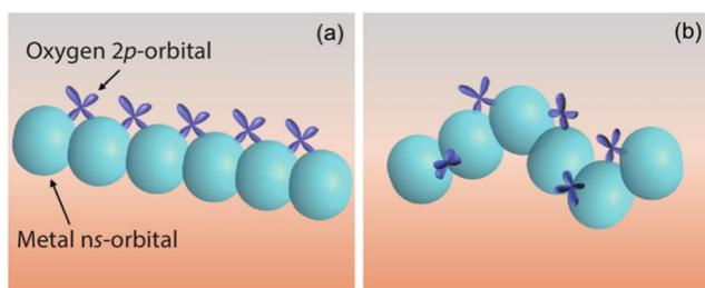
Fig. 1 Carrier transport paths of (a) crystalline and (b) amorphous post-transition-metal oxide semiconductors. Reproduced with permission.<sup>7</sup> Copyright 2024, Springer Nature.
