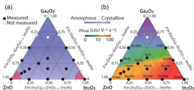
Fig. 2 (a) Crystal morphology distribution and (b) electron transport properties in an  $\text{In}_2\text{O}_3$ – $\text{Ga}_2\text{O}_3$ –ZnO system. In (b), the values outside parentheses denote the electron Hall  $\mu$  ( $\text{cm}^2 \text{ V}^{-1} \text{ s}^{-1}$ ) density, and the values inside parentheses denote the electron concentration ( $\times 10^{18} \text{ cm}^{-3}$ ). Reproduced with permission.<sup>51</sup> Copyright 2024, NPG Asia Materials.
