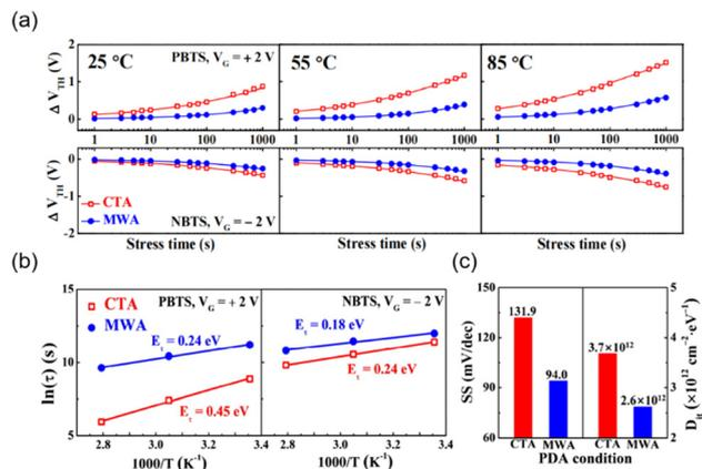
Fig. 18 (a) Time dependence of the  $V_{TH}$  shift under PBTS and NBTS tests at 25, 55, and 85 °C and (b) the  $\ln(\tau)$  as a function of reciprocal temperature ( $1/T$ ) for CTA and MWA processed a-IGZO TFTs. (c) Subthreshold swing and interface trap density. Reproduced with permission.<sup>149</sup> Copyright 2024, K.-W. Park.
