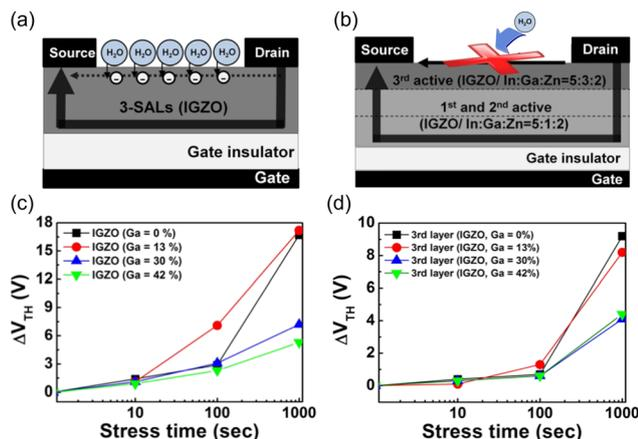
Fig. 10 (a) and (b) Diagram of conventional a-IGZO and a-IGZO TFTs with MSAL. (c) and (d)  $\Delta V_{\text{TH}}$  of a-IGZO and a-IGZO TFTs with MSAL under 1000 s PBS stress. Reprinted with permission from D. J. Kim, Y. S. Rim and H. J. Kim, *ACS Appl. Mater. Interfaces*, 2013, **5**, 4190–4194.<sup>119</sup> Copyright 2024 American Chemical Society.
