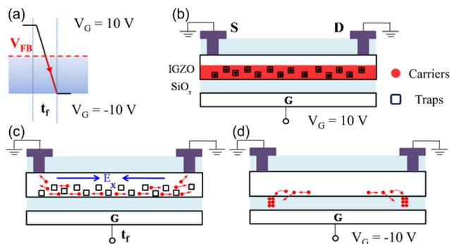
Fig. 20 (a) The diagram of the applied AC bias voltage at the gate. (b) Carrier concentration at positive bias  $V_{FB}$  before AC bias transition. (c) Most carriers deconcentrate during the transition time under flipping E-field. (d) Postponed carriers at the depletion region gain large energy, resulting in hot carrier ejection (HCE) causing damage in the nearby region. Reproduced with permission.<sup>164</sup> Copyright 2024, Applied Physics Letters.
