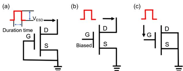
Fig. 6 Connection modes in the TLP pulse test.<sup>100</sup>
