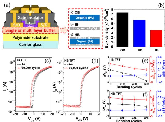
Fig. 23 (a) Diagram of a-IGZO TFTs with buffer layers. The  $\Delta V_{TH}$  of transfer curves before and after 60 000 bending cycles at a bending radius of 1.5 mm for (b) IB TFTs and (c) HB TFTs. Reprinted with permission from K.-L. Han, J.-H. Han, B.-S. Kim, H.-J. Jeong, J.-M. Choi, J.-E. Hwang, S. Oh and J.-S. Park, *ACS Appl. Mater. Interfaces*, 2020, **12**, 3784–3791.<sup>191</sup> Copyright 2024 American Chemical Society.
