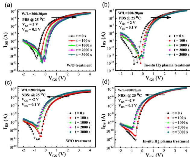
Fig. 9 (a)–(d) Evolution of the transfer curves of a-IGZO TFTs under increasing PBS/NBS duration without and with *in situ* H<sub>2</sub> plasma treatment. Reproduced with permission.<sup>112</sup> Copyright 2024, J. H. Wu, Nanotechnology.
