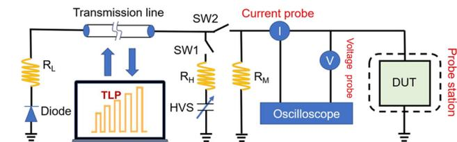
Fig. 5 The setup diagram for ESD reliability characterization.<sup>100</sup>
