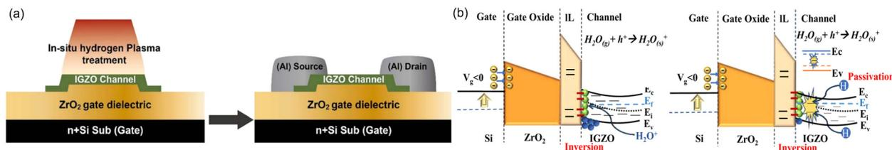
Fig. 8 (a) A cross-sectional schematic of the staggered bottom gate a-IGZO TFTs. (b) Energy band diagrams of a-IGZO TFTs under NBS without and with *in situ* hydrogen plasma treatment. Reproduced with permission.<sup>112</sup> Copyright 2024, J. H. Wu, Nanotechnology.
