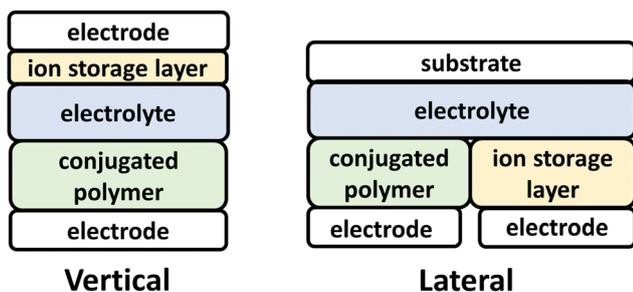
Fig. 3 Vertical (left) and lateral (right) ECD architectures.
