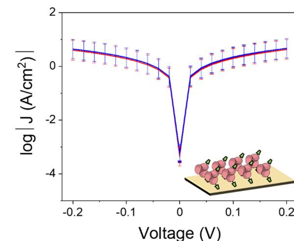
Fig. 6 Semilog plot of current density ( $J$ ) vs. voltage ( $V$ ) for the  $\text{NiAu}^{\text{TS}}/(\text{P})\text{-bPTM-SAM}/\text{GaO}_x/\text{EGaIn}$  junction. Experiments with magnet "up" (red) and "down" (blue).
