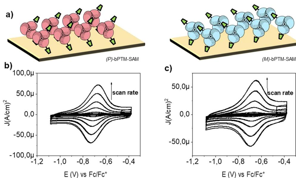
Fig. 5 (a) SAMs schematic representation and cyclic voltammetry of the enantioenriched (b) **(P)-bPTM-SAM** and (c) **(M)-bPTM-SAM** grafted on  $(\text{Au}_{(6\text{nm})}/\text{Ti}_{(2\text{nm})}/\text{quartz})$  at different scan rates. Experimental conditions:  $\text{CH}_2\text{Cl}_2 + 0.2 \text{ M Bu}_4\text{NPF}_6$ ; scan rates: 0.05, 0.1, 0.25, 0.5, 1, 2, 3 and  $4 \text{ V s}^{-1}$ ; Ar atmosphere. WE = SAMs/Au, RE = Ag wire (vs.  $\text{Fc}/\text{Fc}^+$  couple), CE = Pt mesh.
