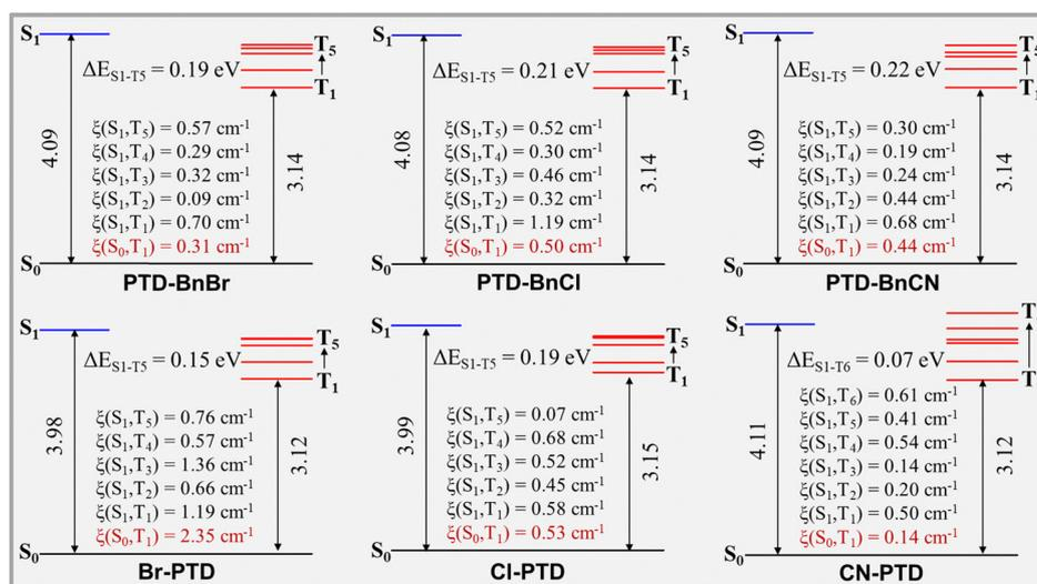
**Fig. 5** Calculated energy level diagrams, spin-orbit coupling (SOC) constants between the involved  $S_n$  and  $T_n$  states of PTD derivatives **PTD-BnBr**, **PTD-BnCl**, **PTD-BnCN**, **Br-PTD**, **Cl-PTD**, and **CN-PTD**, respectively.
