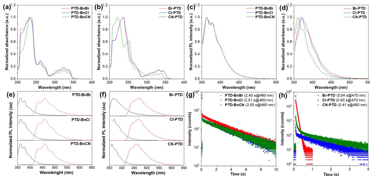
Fig. 2 Photophysical properties of PTD derivatives **PTD-BnBr**, **PTD-BnCl**, **PTD-BnCN**, **Br-PTD**, **Cl-PTD**, and **CN-PTD** in dilute THF solutions ( $10^{-5}$  M): (a) and (b) UV-vis absorption and (c) and (d) steady-state PL spectra at room temperature; (e) and (f) prompt and delayed PL spectra (delay 1 ms) at 77 K; (g) and (h) time-resolved phosphorescence decay curves at 77 K. The excitation wavelength for delayed PL spectra and corresponding decay curves is set to be 340 nm.
