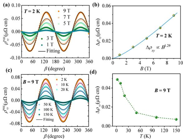
**Fig. 3** (a) The angle-dependent planar Hall resistivity and the corresponding fitting curves under different magnetic fields at 2 K. (b) The magnetic-field-dependent amplitude of the PHE extracted by fitting the curves in (a) *via* theoretical equations. (c) The PHE data and the corresponding fitting curves at various temperatures under 9 T. (d) The temperature-dependent amplitude of the PHE extracted from the fitted curves in (c).
