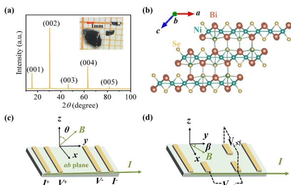
**Fig. 1** (a) The X-ray diffraction pattern of the  $\text{Ni}_3\text{Bi}_2\text{Se}_2$  crystal showing  $(00l)$  ( $l = \text{integer}$ ) diffraction peaks, and the upper inset shows the optical image of the  $\text{Ni}_3\text{Bi}_2\text{Se}_2$  single crystal. (b) The schematic crystal structure of  $\text{Ni}_3\text{Bi}_2\text{Se}_2$ . (c) The device configuration for out-of-plane transport measurement. (d) The schematic of the experimental configuration for the PHE and PAMR measurement.
