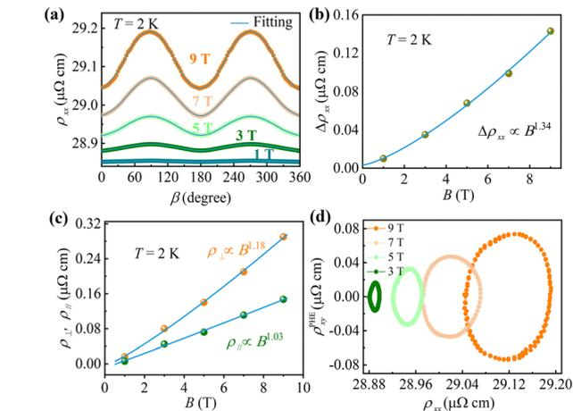
**Fig. 4** (a) The angle dependence of planar resistivity under different magnetic fields at  $T = 2$  K. (b) Magnetic field dependence of resistivity amplitude extracted from the fitting curves in (a), and the solid curve is the power law fitting result. (c) Magnetic field dependence of  $\rho_{\perp}$  and  $\rho_{\parallel}$  at 2 K. The blue line represents the power law fitting results. (d) Parametric plots of the planar Hall resistivity and planar resistivity showing the orbits at 2 K.
