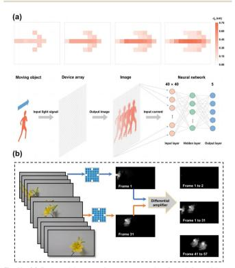
Fig. 11 (a) Projected images of an arrow moving from left to right at various times in a 10 imes 10 neuromorphic photosensor array and a schematic diagram of the neuromorphic photosensor array in conjunction with a neural network. Reproduced with permission.<sup>27</sup> Copyright 2024, Wiley-VCH. (b) Illustration of motion detection with the BTBTT6-synbased synaptic OPT arrays. Reproduced with permission.<sup>53</sup> Copyright 2023, Springer Nature.
