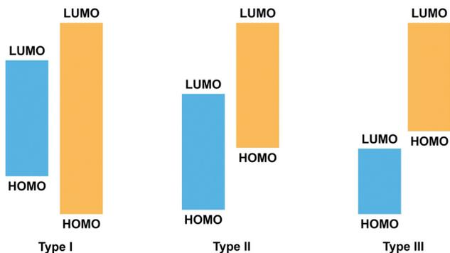
Fig. 5 Three types of heterojunctions are classified according to bandgap alignment. Type I: straddling gap; type II: staggered gap; and type III: broken gap.
