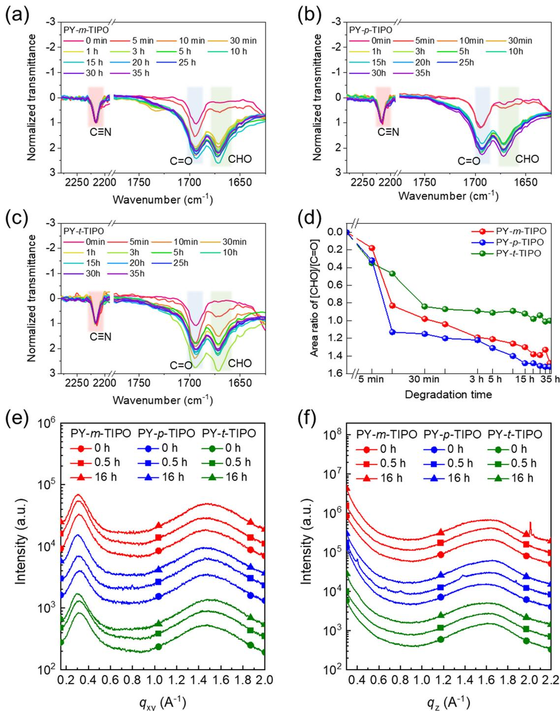
Fig. 4 The normalized FT-IR spectra at cyanide transmittance ( $2216\text{ cm}^{-1}$ ) of films based on (a) PY-*m*-TIPO, (b) PY-*p*-TIPO and (c) PY-*t*-TIPO in 0.1 M TFA during the degradation procedure. (d) The degradation rate defined by the ratio of integrated areas of aldehyde and ketone peaks. (e) In-plane and (f) out-of-plane line-cut profiles from 2D-GIWAXS patterns.
