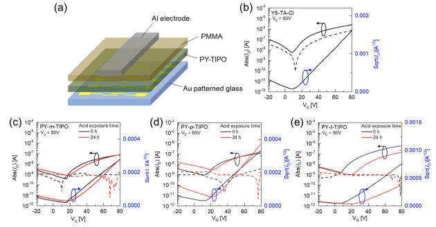
Fig. 5 (a) Top-gate bottom-contact (TGBC) OTFT device structure. Transfer characteristics of (b) Y5-TA-Cl, (c) PY-m-TIPO, (d) PY-p-TIPO and (e) PY-t-TIPO-based OTFTs before and after exposure to acid vapor for 24 h (V<sub>D</sub>: drain-source voltage = 80 V, I<sub>D</sub>: drain-source current; V<sub>G</sub>: gate-source voltage)
