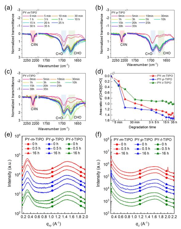
Fig. 4 The normalized FT-IR spectra at cyanide transmittance (2216 cm<sup>-1</sup>) of films based on (a) PY-m-TIPO, (b) PY-p-TIPO and (c) PY-t-TIPO in 0.1 M TFA during the degradation procedure. (d) The degradation rate defined by the ratio of integrated areas of aldehyde and ketone peaks. (e) In-plane and (f) out-of-plane line-cut profiles from 2D-GIWAXS patterns.
