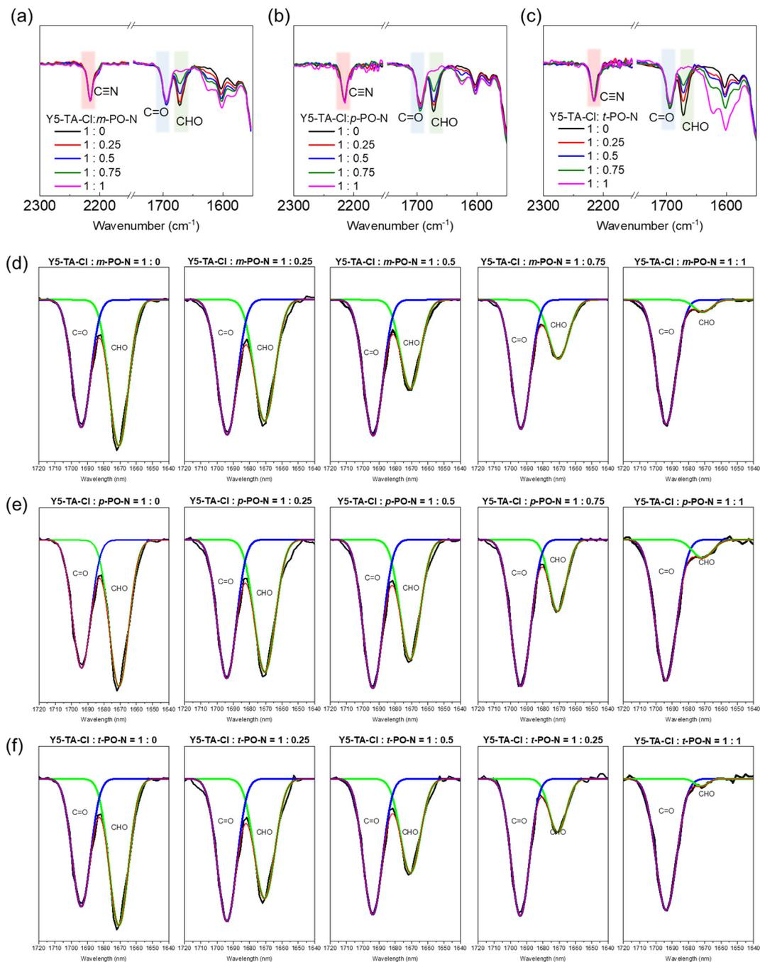
Fig. 2 The normalized FT-IR spectra of Y5-TA-Cl with (a) *m*-PO-N, (b) *p*-PO-N, and (c) *t*-PO-N annealed films in various stoichiometric ratios (Y5-TA-Cl: PO-N = 1 : 0, 1 : 0.25, 1 : 0.5, 1 : 0.75, 1 : 1). The deconvoluted FT-IR spectra by Gaussian fitting of Y5-TA-Cl with (d) *m*-PO-N, (e) *p*-PO-N, and (f) *t*-PO-N.
