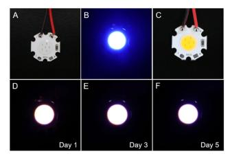
Fig. 5 (A)-(C) Fabrication of while light-emitting device based on blue LEDs by coating a TPP-C2(R)/Dye-O film. (D)-(F) Exhibition of white light emission by the device in 5 days.
