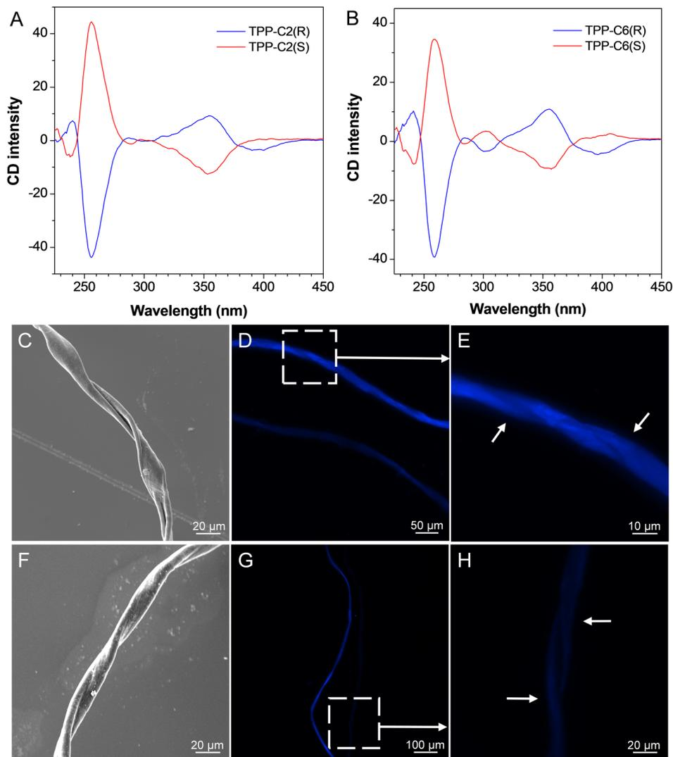
Fig. 2 CD spectra of (A) TPP-C2(R) and TPP-C2(S) and (B) TPP-C6(R) and TPP-C6(S) in THF. SEM and fluorescence images of self-assemblies formed by (C)–(E) TPP-C6(R) and (F)–(H) TPP-C6(S) in a  $\text{CHCl}_3/\text{CH}_3\text{CN}$  ( $v/v = 1:1$ ) mixture.
