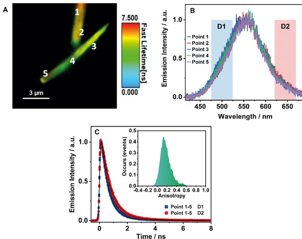
Fig. 7 (A) FLIM of **BTIA-HOF** crystals. (B) Normalized emission spectra of **BTIA-HOF** at different points of the crystals. (C) Fluorescence emission decays of **BTIA-HOF** crystals in the selected spectral range using two different filters (D1 and D2 in (B)). The solid lines are from the best fit using a multiexponential function. Inset shows the histogram of the emission anisotropy for **BTIA-HOF** crystals. The excitation wavelength was 371 nm.
