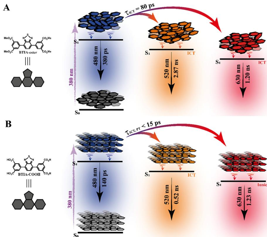
**Scheme 2** Proposed photodynamic schemes for **BTIA-ester** (A) and **BTIA-HOF** (B) in solid state, in which ICT is the intramolecular charge-transfer process and PT is the intermolecular proton-transfer reaction. The emission wavelengths were chosen based on the time-resolved spectra and the contributions obtained in the fit of the picosecond emission decays. The schemes are not to scale.
