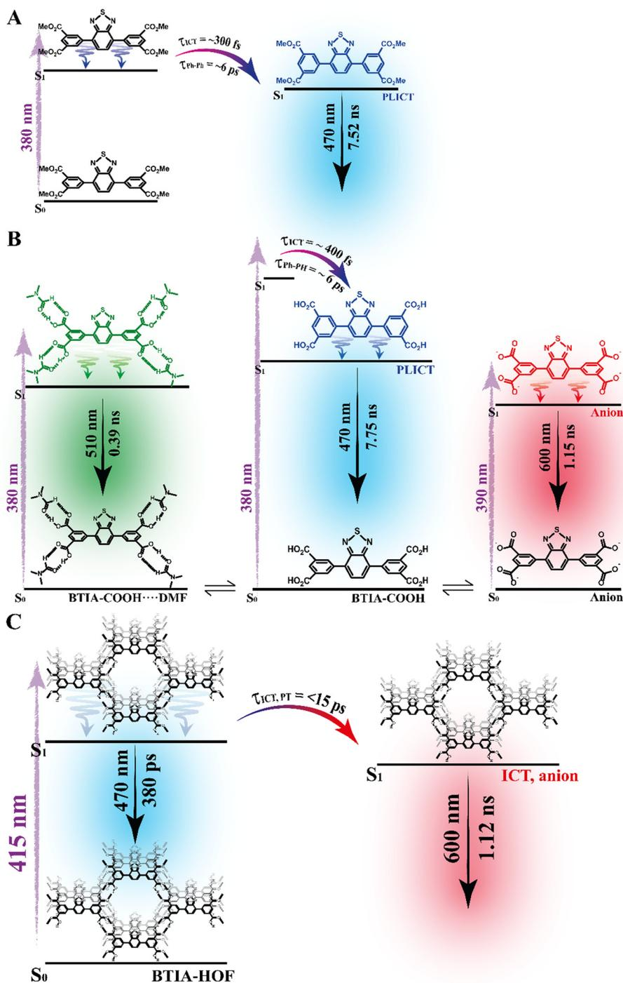
**Scheme 1** Proposed photodynamic schemes for **BTIA-ester** (A), **BTIA-COOH** (B) and **BTIA-HOF** (C) in a DMF solution or suspension, in which PLICT is the planarized intramolecular charge-transfer process,  $\tau_{ICT}$  is the ICT reaction time,  $\tau_{Ph-Ph}$  is the time of the twisting motions of the phenyl rings, and  $\tau_{PT}$  is the time of the intermolecular PT process. The scheme is not to scale.
