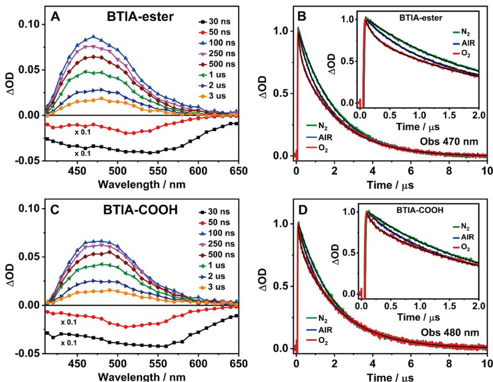
Fig. 4 Time-resolved transient absorption spectra (TAS) of **BTIA-ester** (A) and **BTIA-COOH** (C) in a DMF solution at different delay times. Transient absorption decays of **BTIA-ester** (B) and **BTIA-COOH** (D) in DMF solutions probed at 470 nm and 480 nm under different atmospheric conditions: air (blue), oxygen (red), and nitrogen (green). The excitation wavelength was 355 nm.
