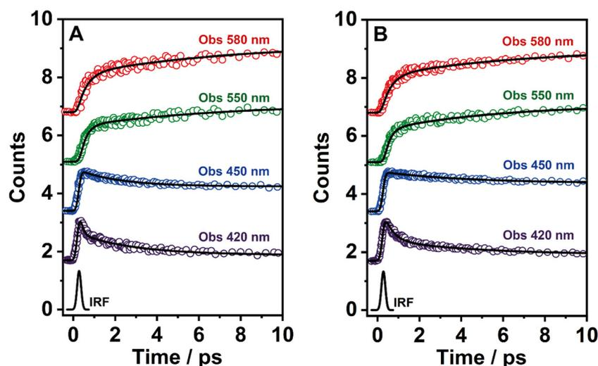
Fig. 3 Representative fs-emission transients of (A) **BTIA-ester** and (B) **BTIA-COOH** in a DMF solution. The samples were excited at 360 nm and recorded at the indicated wavelengths. The solid lines are from the best multiexponential fit and the IRF is the instrumental response function (220 fs).
