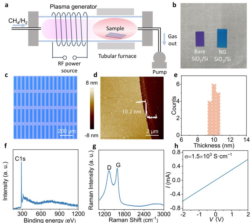
**Fig. 1** NG electrodes grown by PECVD. (a) Schematic diagram of the PECVD system. (b) Optical image of bare  $\text{SiO}_2/\text{Si}$  and NG film grown on  $\text{SiO}_2/\text{Si}$ , respectively. (c) Optical image of the NG electrode array. (d) AFM image of the edge of the NG electrode. (e) Thickness statistics of 15 NG electrodes. (f) XPS spectra of the NG electrode. (g) Raman spectra of the NG electrode. (h)  $I$ - $V$  characteristic of the NG electrode.
