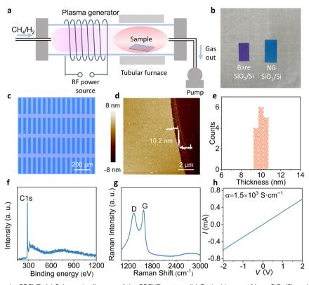
Fig. 1 NG electrodes grown by PECVD. (a) Schematic diagram of the PECVD system. (b) Optical image of bare  $SiO_2/Si$ , and NG film grown on  $SiO_2/Si$ , respectively. (c) Optical image of the NG electrode array. (d) AFM image of the edge of the NG electrode. (e) Thickness statistics of 15 NG electrodes. (f) XPS spectra of the NG electrode. (g) Raman spectra of the NG electrode. (h) I-V characteristic of the NG electrode.
