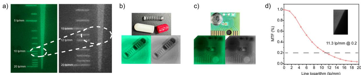
**Fig. 4** (a) The spatial resolution of X-ray imaging for the **TPPOMnBr<sub>2</sub>**-based film scintillator. X-ray images of a metallic spring in the capsule (b) and circuit board (c) based on the **TPPOMnBr<sub>2</sub>**-based film scintillator. (d) MTF curve of the **TPPOMnBr<sub>2</sub>**-based film scintillator measured by the slanted-edge method.
