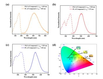
Fig. 2 1 (a), 2 (b) and 3 (c) PLE and PL spectra at room temperature. The solid lines are the emission spectra at different excitation wavelengths. The dashed lines are the excitation spectra at different emission wavelengths. (d) CIE chromaticity coordinates corresponding to 1, 2 and 3. Inset: Photographs of the compounds under UV light.
