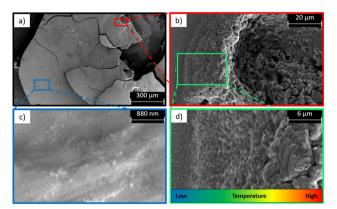
Fig. 7 Representative SEM images of the YVO<sub>4</sub>:20%Yb<sup>3+</sup>,2%Er<sup>3+</sup> pellet (a), showing the laser-treated (b), untreated (c) and surroundings of the lasertreated (d) regions
