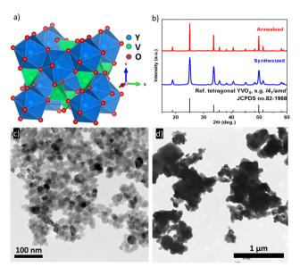
Fig. 2 (a) 3D representation of the tetragonal YVO<sub>4</sub> (I4<sub>1</sub>/amd) structure. (b) Comparison of the PXRD patterns with the reference data. (c) and (d) Representative TEM images of the hydrothermally synthesized nanomaterial (c) with the sample annealed at high-temperature (d).
