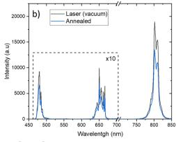
Fig. 6 (a) Differences in UC intensities between the two samples: YVO<sub>4</sub>:20%Yb<sup>3+</sup>,2%Er<sup>3+</sup> annealed and after the laser treatment under vacuum at 0.9 kW cm<sup>-2</sup>. (b) Differences in the UC intensities between the two samples: YVO<sub>4</sub>:20%Yb<sup>3+</sup>,0.5%Tm<sup>3+</sup> annealed and after the laser treatment under vacuum at 1.5 kW cm<sup>-2</sup>
