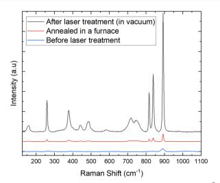
Fig. 5 Raman spectra of the hydrothermally synthesized YVO<sub>4</sub>:Yb $^{3+}$ – Tm $^{3+}$ , before and after laser treatment under vacuum and after standard annealing in a furnace.
