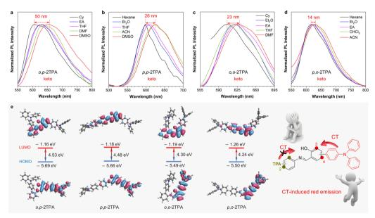
Fig. 3 Normalized PL spectra of (a) o,p-2TPA, (b) p,p-2TPA, (c) o,o-2TPA, and (d) p,o-2TPA in different solvents with varying polarities. (e) Frontier molecular orbitals of the four isomers and the energy gaps between the HOMO and LUMO.
