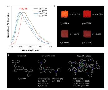
Fig. 4 (a) Normalized PL spectra of the four isomers as solids.  $\lambda_{ex}$  = 429 nm for o,p-2TPA, 476 nm for p,p-2TPA, 405 nm for o,o-2TPA, and 466 nm for p,o-2TPA. (b) Fluorescence photographs and quantum yields of the four isomers. (c) Chemical structure, twist conformation, and intermolecular interactions based on the single-crystal structure of o,p-2TPA
