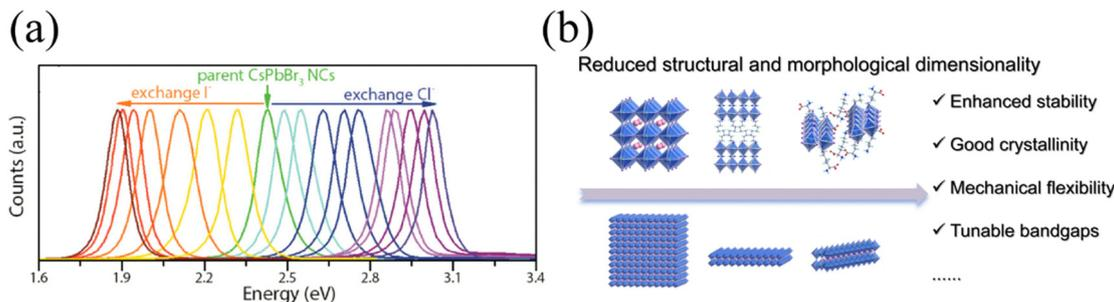
Fig. 2 (a) Bandgaps of MHPs (CsPbBr<sub>3</sub> nanocrystals) can be tuned by changing halide components. Reproduced with permission.<sup>17</sup> Copyright 2015, ACS. (b) Optical and electrical properties can be tuned by the tunable dimensionality at the structural and morphological level of MHPs. Reproduced with permission.<sup>18</sup> Copyright 2021, ACS.
