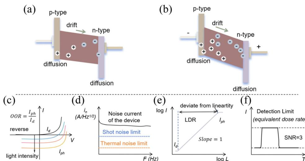
Fig. 1 Schematic illustration of the energy diagram of P-I-N photodiodes without bias (a) and under bias conditions (b). Schematic of the parameters influenced by  $I_d$  in photodiodes for light sensing and direct X-ray detection. (c) On-off ratio (OOR). (d) Noise current ( $i_n$ ). (e) Linear dynamic range (LDR). (f) Detection limit.
