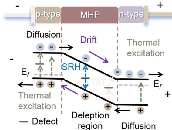
Fig. 3 The typical components and generation mechanisms of dark current in MHPPDs.
