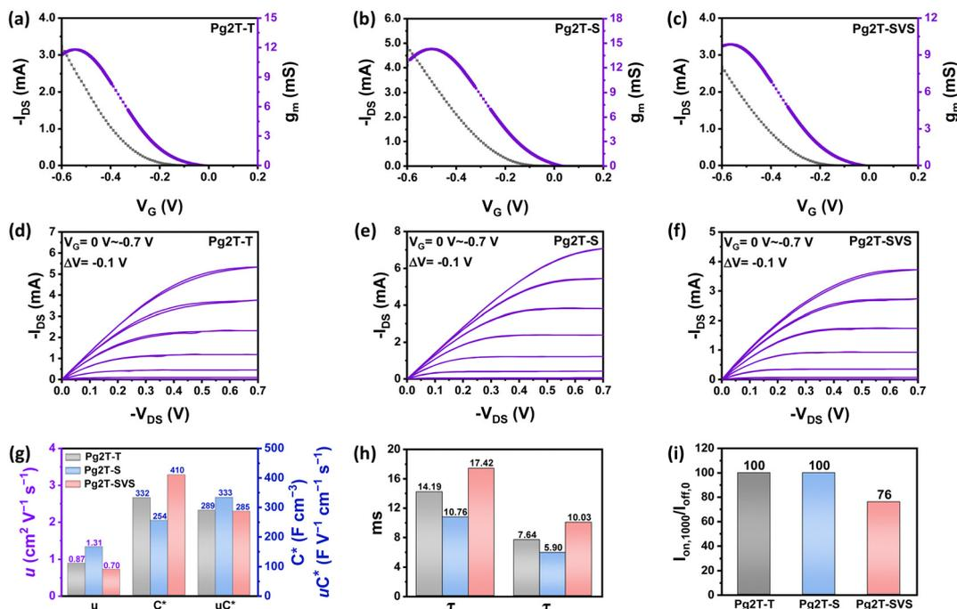
Fig. 4 The typical output, transfer and transconductance curves of (a) and (d) Pg2T-T, (b) and (e) Pg2T-S, and (c) and (f) Pg2T-SVS based OECTs. (g) Calculated  $\mu C^*$ ,  $\mu$ , and  $C^*$ , (h)  $\tau_{on}/\tau_{off}$  response time, and (i) retained ON current after 1000 cycles of Pg2T-T, Pg2T-S, and Pg2T-SVS based OECTs.
