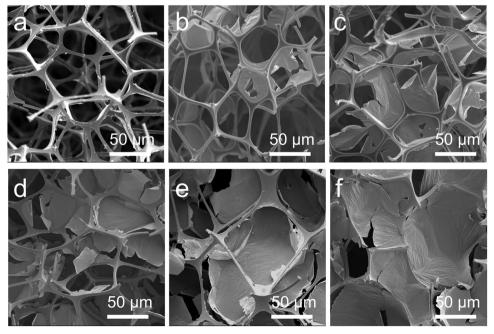
Fig. 3 The microscopic morphology of GCNP sponges prepared with different GO concentrations. (a) SEM image of the melamine sponge. (b) – (f) SEM images of the GCNP with different concentrations of GO ink (0.5, 1.0, 2.0, 3.0, 4.0 mg mL<sup>-1</sup>).
