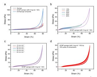
Fig. 4 Mechanical properties of the GCNP sponge (with 3 mg mL<sup>-1</sup> GO concentration). (a) Comparison of the compression behavior among the sponge, GO/Sponge composite prepared by immersion method, and GCNP sponge obtained by direct writing. (b) and (c) Compression loading-unloading curves of GCNP sponge at different compressive strains and different compression rates. (d) Cyclic loading-unloading curves of GCNP sponge at compressive strain of 80%
