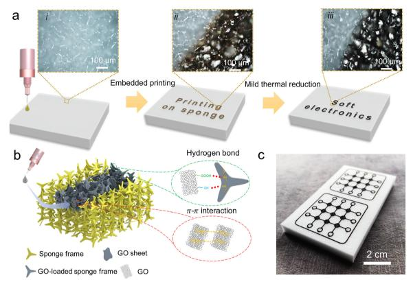
Fig. 1 Preparation and patterning of GCNP sponge by embedded printing. (a) Schematic diagram of the fabrication process and the corresponding microscopic images of the internal structure of the sponge. (b) Schematic diagram of the assembly mechanism of GO within the sponge. (c) Top-view optical image of the printed GCNP sponge.
