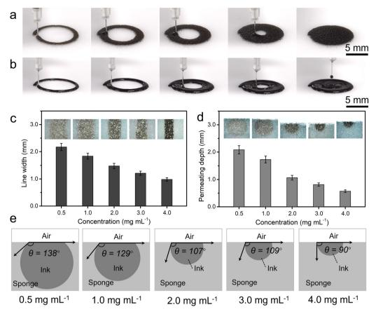
Fig. 2 Direct-write printing processes and morphologies of the GCNP. (a) Printing processes of GO ink with low concentration (1 mg mL<sup>-1</sup>). (b) Printing processes using GO ink of high concentration (3 mg mL<sup>-1</sup>). (c) The relationship between the concentration of GO ink and line width of GCNP from top view. (d) Penetration depth of the GCNP in the sponge from side view. (e) Schematic representation of the penetration morphologies of GCNP with different concentrations of GO ink.
