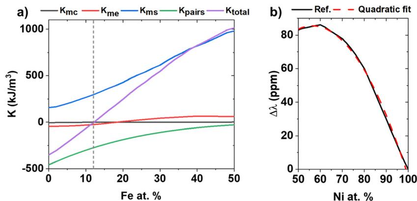
Fig. 4 (a) Dependency of the different magnetic anisotropies with respect to Fe content (at%). The dashed line at Fe 12 at% indicates the change of sign in  $K_{\text{total}}$ . (b) Excess magnetostriction ( $\Delta\lambda$ ) obtained from the references (black)<sup>20</sup> with its quadratic fit (dashed-red).
