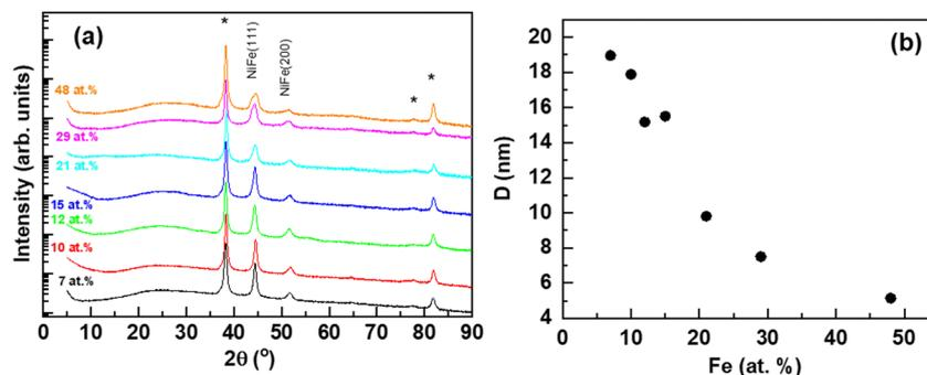
Fig. 3 (a) XRD diffraction patterns for different electrodeposited  $\text{Ni}_{100-x}\text{Fe}_x$  layers. Curves have been vertically shifted for clarity. \* is used to indicate peaks related to the Au layer. (b) Coherent domain size ( $D$ ) inferred from Scherrer's equation as a function of the Fe content.
