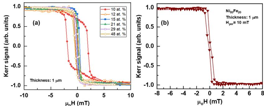
Fig. 2 (a) MOKE hysteresis loops for 1  $\mu\text{m}$  thick  $\text{Ni}_{100-x}\text{Fe}_x$  layers with different Fe contents indicated in the label. (b) MOKE hysteresis loop for a 1  $\mu\text{m}$  thick  $\text{Ni}_{80}\text{Fe}_{20}$  layer deposited under an applied magnetic field of 10 mT perpendicular to the sample plane.
