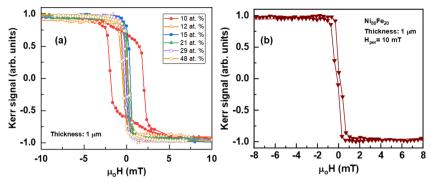
Fig. 2 (a) MOKE hysteresis loops for 1  $\mu$ m thick Ni<sub>100-x</sub>Fe<sub>x</sub> layers with different Fe contents indicated in the label. (b) MOKE hysteresis loop for a 1  $\mu$ m thick Ni<sub>80</sub>Fe<sub>20</sub> layer deposited under an applied magnetic field of 10 mT perpendicular to the sample plane
