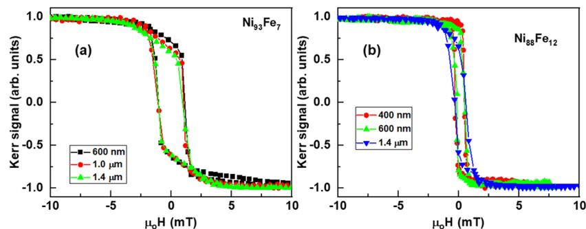
Fig. 1 (a) MOKE hysteresis loops for  $\text{Ni}_{93}\text{Fe}_7$  layers with different thicknesses: (■) 600 nm, (●) 1  $\mu\text{m}$ , and (▲) 1.4  $\mu\text{m}$ . (b) MOKE hysteresis loops for  $\text{Ni}_{88}\text{Fe}_{12}$  layers with different thicknesses: (●) 400 nm, (▲) 600 nm, and (▼) 1.4  $\mu\text{m}$ .
