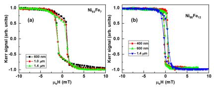
Fig. 1 (a) MOKE hysteresis loops for Ni<sub>93</sub>Fe<sub>7</sub> layers with different thicknesses: (■) 600 nm, (●) 1 μm, and (▲) 1.4 μm. (b) MOKE hysteresis loops for Ni<sub>88</sub>Fe<sub>12</sub> layers with different thicknesses: (●) 400 nm, (▲) 600 nm, and (▼) 1.4 μm.
