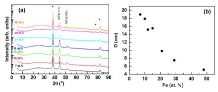
Fig. 3 (a) XRD diffraction patterns for different electrodeposited  $Ni_{100-x}Fe_x$  layers. Curves have been vertically shifted for clarity. \* is used to indicate peaks related to the Au layer. (b) Coherent domain size (D) inferred from Scherrer's equation as a function of the Fe content.
