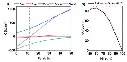
Fig. 4 (a) Dependency of the different magnetic anisotropies with respect to Fe content (at%). The dashed line at Fe 12 at% indicates the change of sign in  $K_{\text{total}}$ . (b) Excess magnetostriction ( $\Delta\lambda$ ) obtained from the references (black)<sup>20</sup> with its quadratic fit (dashed-red).
