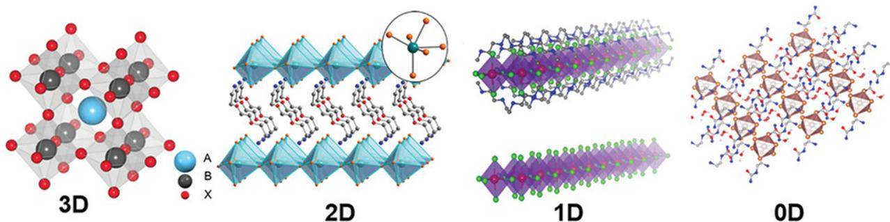
Fig. 1 Schematic diagram of the atomic level structures of 0D-3D MHP.<sup>93</sup> Copyright 2021, The Authors. Advanced Science published by Wiley-VCH GmbH.
