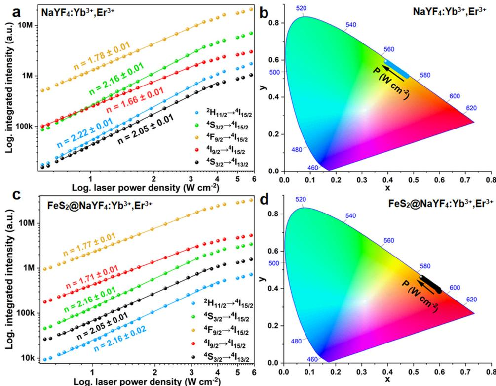
Fig. 4 Integrated luminescence intensity as a function of laser power density for the  $\text{NaYF}_4:\text{Yb}^{3+},\text{Er}^{3+}$  NPs (a) and  $\text{FeS}_2@\text{NaYF}_4:\text{Yb}^{3+},\text{Er}^{3+}$  NC (c). CIE diagrams for the NPs (b) and NC (d) showing the color coordinates as a function of laser power density.
