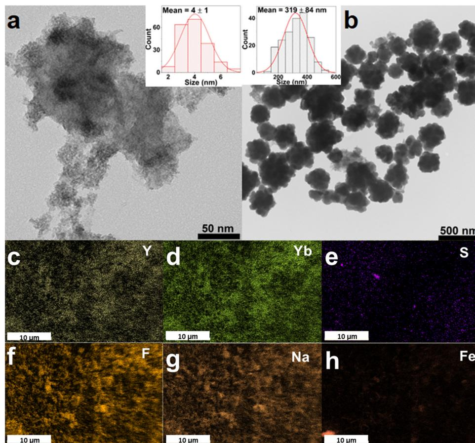
Fig. 2 The representative TEM images of the FeS<sub>2</sub> NPs (a) and FeS<sub>2</sub>@NaYF<sub>4</sub>:Yb<sup>3+</sup>,Er<sup>3+</sup> NC (b); the insets show histograms of the NPs and NC size distribution. The EDX mapping of elements in the FeS<sub>2</sub>@NaYF<sub>4</sub>:Yb<sup>3+</sup>,Er<sup>3+</sup> NC, *i.e.*, Y (c), Yb (d), S (e), F (f), Na (g), Fe (h).
