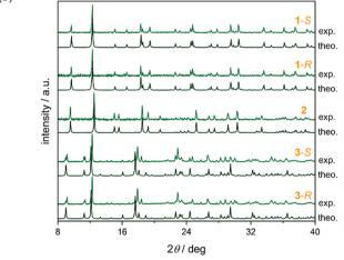
Fig. 3 The air- and thermal stability as well as phase purity of obtained materials: (a) the TG curves of  $\mathbf{1}$ -R and  $\mathbf{3}$ -R, and (b) the comparison of experimental (T=300 K) powder X-ray diffraction patterns of  $\mathbf{1}$ -S,  $\mathbf{1}$ -R,  $\mathbf{2}$ ,  $\mathbf{3}$ -S, and  $\mathbf{3}$ -R with the patterns calculated from the respective structural models obtained from the SC-XRD structural analysis (T=100 K).
