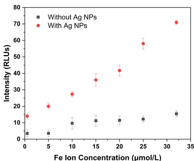
Fig. 7 Calibration curves for Fe ion concentration with and without the incorporation of TA-Ag 93 NPs. The normal Fe ion level for adults is  $10\text{--}32 \mu\text{mol L}^{-1}$  of blood. Without TA-Ag 93 NPs, the luminol- $\text{H}_2\text{O}_2$  system exhibits weak luminescence. The introduction of TA-Ag 93 NPs reduced the limit of detection and enhanced the intensity at higher concentrations, facilitating clearer observations.
