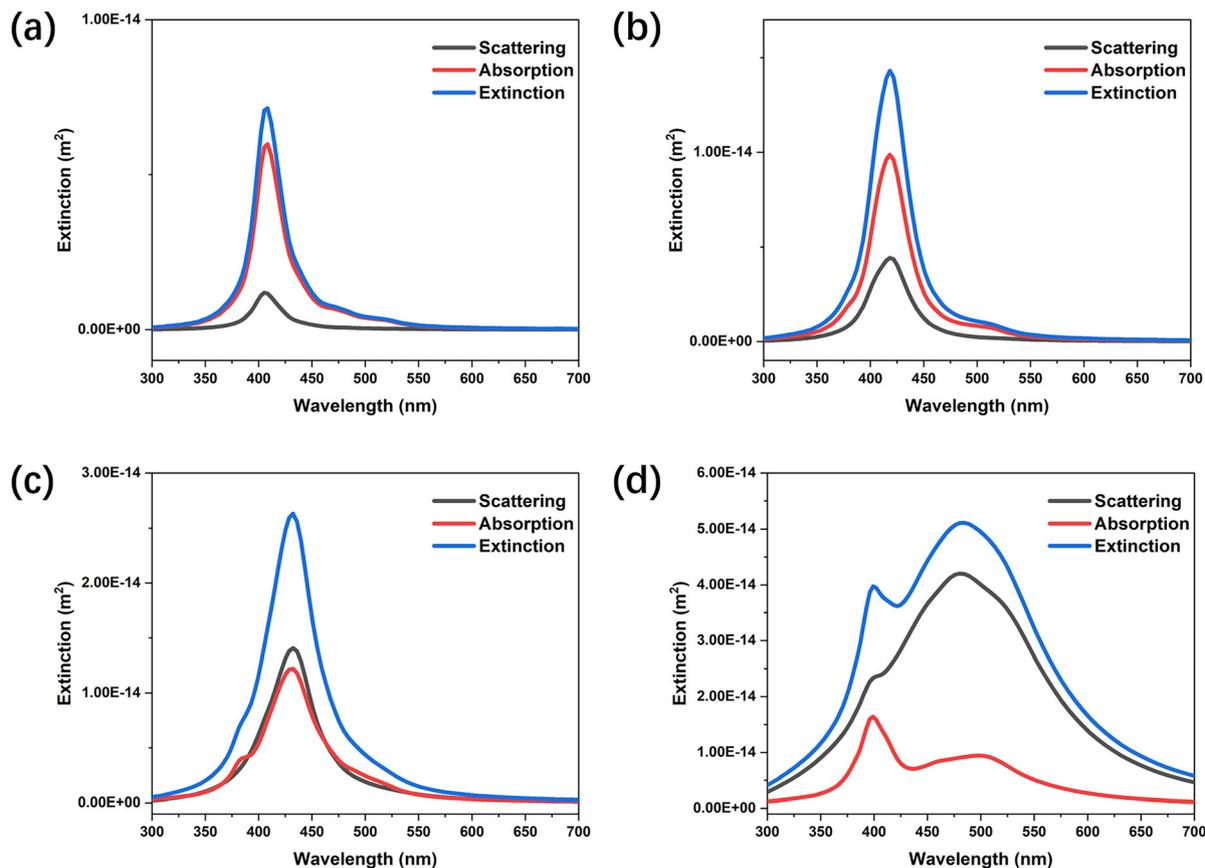
Fig. 5 (a)–(d) The extinction cross-sections of TA-Ag 31, 41, 53, 93 modelled by FDTD. The scattering cross-sections overtake the absorption cross-section as the sizes increase to 53 nm.
