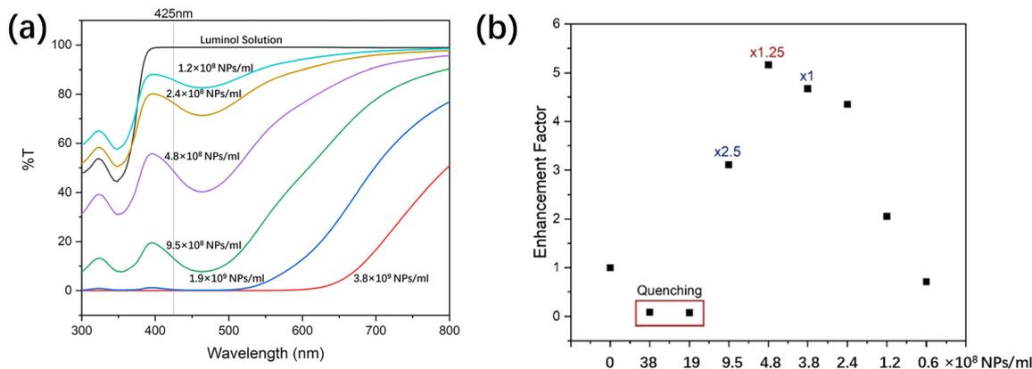
Fig. 6 (a) Light transmittance spectra of varying concentrations of TA-Ag 93 solutions. As the NPs solutions become more concentrated, the transmittance of blue light decreases, resulting in self-absorption and reduced emission intensity. (b) CL intensity spectra of luminol CL reactions enhanced by different concentrations of TA-Ag 93 solutions. The optimised concentration is x1.25 times more concentrated TA-Ag 93 solutions.
