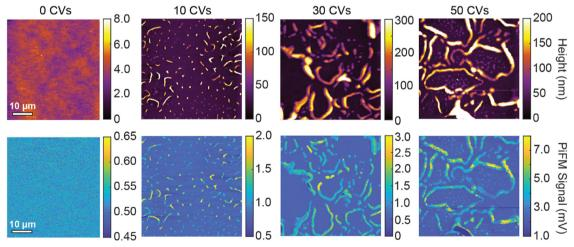
Fig. 4 AFM topography and PiFM images of a RRa P3HT thin film upon increasing numbers of CVs performed in aqueous 100 mM KTFSI after a 40 s -0.5 V (vs. Ag/AgCI) dedoping step.  $50 \times 50$   $\mu$ m AFM topography and PiFM images are collected of an undoped RRa P3HT thin film, as well as RRa P3HT thin films that underwent 0, 10, 30, and 50 CVs.
