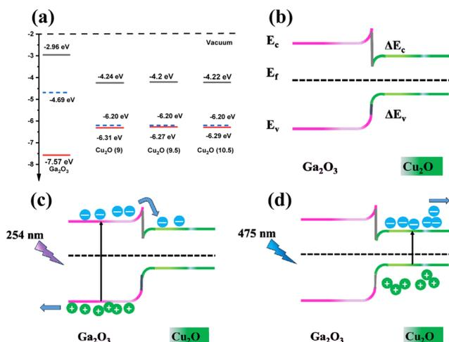
Fig. 6 Energy band structures of Ga<sub>2</sub>O<sub>3</sub> and Cu<sub>2</sub>O prepared at different pH values (a) before and (b) contact. The schematic diagram of carrier transport of Cu<sub>2</sub>O/Ga<sub>2</sub>O<sub>3</sub> heterojunction under (c) 254 (d) 475 nm illuminations.
