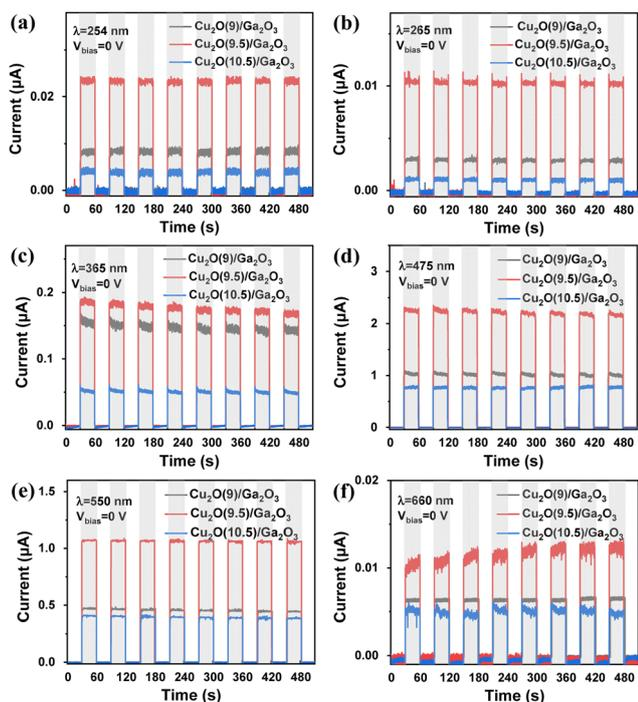
Fig. 4  $I$ - $t$  cycling curves at zero bias for  $\text{Cu}_2\text{O}/\text{Ga}_2\text{O}_3$  heterojunction PDs with  $\text{Cu}_2\text{O}$  at different pH values under (a) 254, (b) 265, (c) 365, (d) 475, (e) 550 and (f) 660 nm illuminations with  $P = 4 \text{ mW cm}^{-2}$ .
