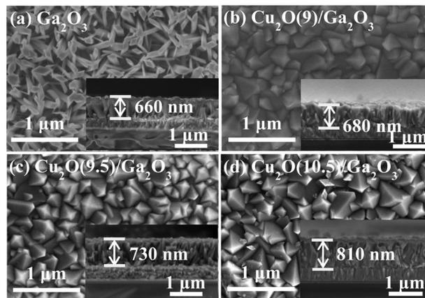
Fig. 1 The top-view and cross-sectional view of SEM images of (a)  $\text{Ga}_2\text{O}_3$  NRs and (b)  $\text{Cu}_2\text{O}(9)/\text{Ga}_2\text{O}_3$ , (c)  $\text{Cu}_2\text{O}(9.5)/\text{Ga}_2\text{O}_3$  and (d)  $\text{Cu}_2\text{O}(10.5)/\text{Ga}_2\text{O}_3$ .
