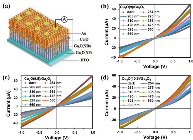
Fig. 3 (a) Schematic diagram of the PD structure of  $\text{Cu}_2\text{O}/\text{Ga}_2\text{O}_3$  PDs. Dark-state and different wavelengths light illuminations  $I$ - $V$  curves for (b)  $\text{Cu}_2\text{O}(9)/\text{Ga}_2\text{O}_3$  PDs, (c)  $\text{Cu}_2\text{O}(9.5)/\text{Ga}_2\text{O}_3$  PDs and (d)  $\text{Cu}_2\text{O}(10.5)/\text{Ga}_2\text{O}_3$  PDs under an optical power density of  $4 \text{ mW cm}^{-2}$  illumination.
