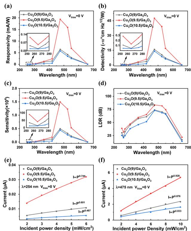
Fig. 5 Performance parameters of (a)  $R$ , (b)  $D^*$ , (c)  $S$  and (d) LDR of  $\text{Cu}_2\text{O}/\text{Ga}_2\text{O}_3$  heterojunction PDs with  $\text{Cu}_2\text{O}$  prepared at different pH values at 0 V bias voltage under solar-blind UV, UV and visible light illuminations with  $4 \text{ mW cm}^{-2}$  optical power density. Photocurrent under (e) 254 and (f) 475 nm illuminations of  $\text{Cu}_2\text{O}/\text{Ga}_2\text{O}_3$  heterojunction PDs at different optical power densities.
