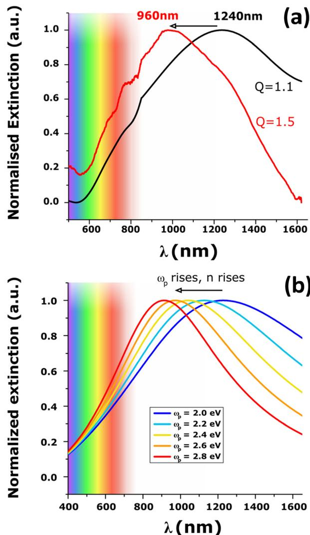
Fig. 3 (a) Normalized extinction spectra of PEDOT NPs (diameter 90 nm, height 65 nm) before (black curve) and after (red curve) acid treatment. (b) Simulation of the effect of plasma frequency, *i.e.* the density of charge-carriers, on the LSPR wavelength calculated using the Drude model and using  $\omega_p$  values from 2 eV to 2.8 eV.
