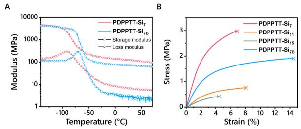
Fig. 4 Mechanical properties of PDPPT-Si<sub>7</sub>. (A) DMA traces of PDPPTT-Si<sub>7</sub> and PDPPTT-Si<sub>7</sub> showing storage and loss moduli as a function of temperature. A heating rate of 3 °C min<sup>-1</sup> at a frequency of 1 Hz and a strain of 0.1% were applied. (B) Stress-strain curves for PDPPTT-Si<sub>7</sub>, PDPPTT-Si<sub>11</sub>. PDPPTT-Si<sub>15</sub>, and PDPPTT-Si<sub>7B</sub> obtained from tensile tests on free-standing films.
