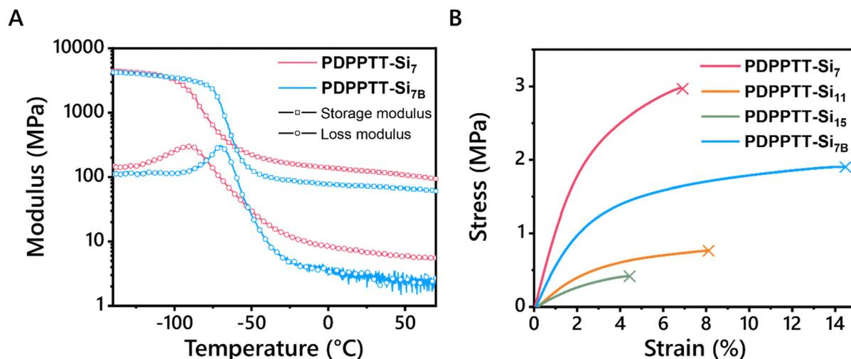
Fig. 4 Mechanical properties of **PDPPT-Si<sub>n</sub>**. (A) DMA traces of **PDPPT-Si<sub>7</sub>** and **PDPPT-Si<sub>7B</sub>** showing storage and loss moduli as a function of temperature. A heating rate of 3 °C min<sup>−1</sup> at a frequency of 1 Hz and a strain of 0.1% were applied. (B) Stress–strain curves for **PDPPT-Si<sub>7</sub>**, **PDPPT-Si<sub>11</sub>**, **PDPPT-Si<sub>15</sub>**, and **PDPPT-Si<sub>7B</sub>** obtained from tensile tests on free-standing films.
