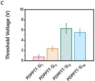
Fig. 5 Charge carrier mobilities (A), on/off ratios (B) and threshold voltages (C) of BGTC OFETs fabricated from PDPPTT-Sin
