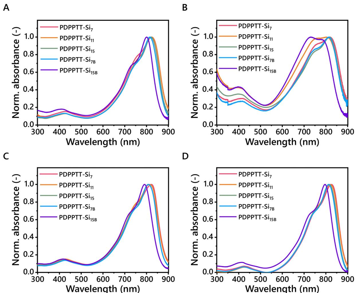
Fig. 2 UV-Vis spectra of PDPPTT-Si<sub>n</sub> in (A) CHCl<sub>3</sub>, (B) *o*-DCB, (C) methylcyclohexane and (D) toluene ( $l = 1$  mm,  $c = 0.08$  mg mL<sup>-1</sup>).
