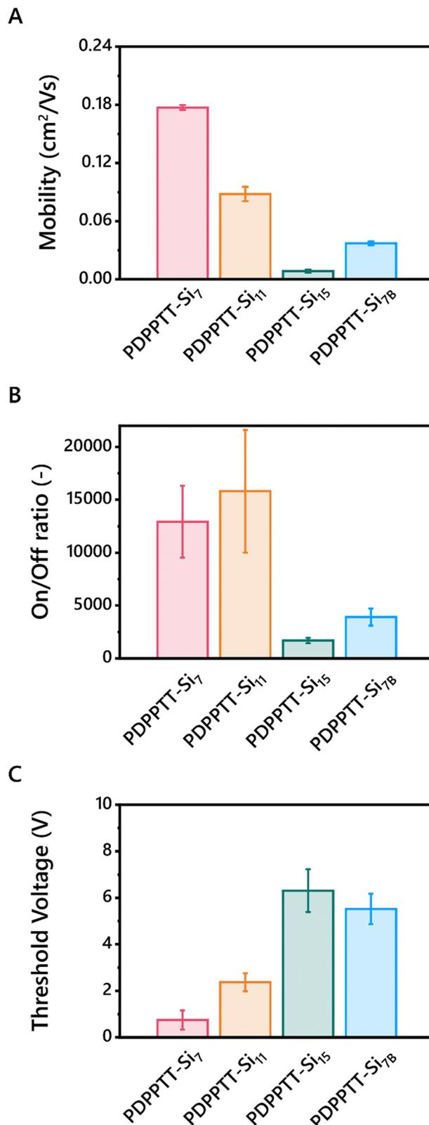
Fig. 5 Charge carrier mobilities (A), on/off ratios (B) and threshold voltages (C) of BGTC OFETs fabricated from PDPPTT-Si<sub>n</sub>.
