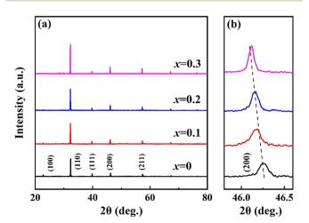
Fig. 2 (a) XRD pattern of (0.8 - x)BNT-BZT-xNN ceramics. (b) Partial enlargement of 45.8-46.6°.
