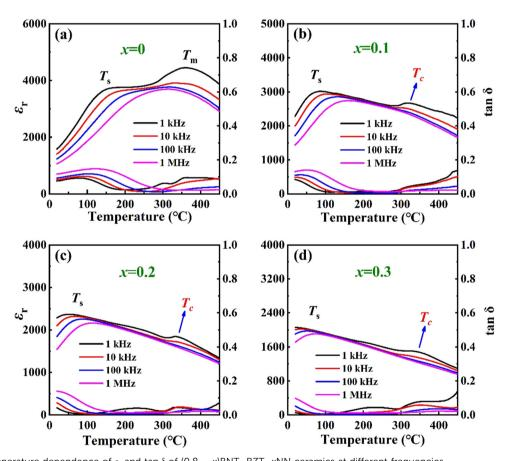
Fig. 4 (a)–(d) Temperature dependence of  $\varepsilon_r$  and  $\tan \delta$  of (0.8 – x)BNT–BZT–xNN ceramics at different frequencies.
