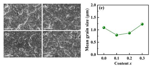
Fig. 3 (a)–(d) SEM images and (e) mean grain size with the increase of content x of (0.8 - x)BNT-BZT-xNN ceramics.
