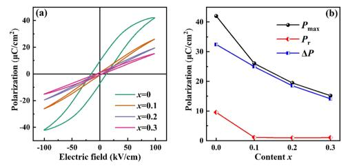
(a) The bipolar P-E loops at 100 kV cm $^{-1}$  of (0.8 - x)BNT-BZT-xNN ceramics and (b)  $P_{\text{max}}$ ,  $P_{\text{r}}$  and  $\Delta P$  ( $P_{\text{max}}-P_{\text{r}}$ ) as a function of x content.
