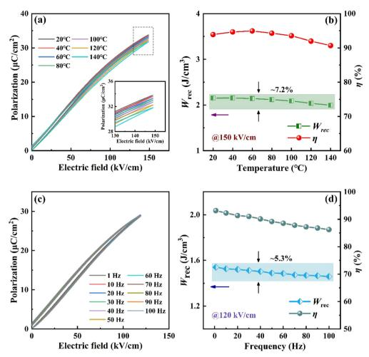
Fig. 8 Unipolar P-E loops and energy storage properties of 0.7BNT-0.2BZT-0.1NN ceramic at (a) and (b) different temperatures and (c) and (d) different frequencies. The inset in (a) shows a localized magnified view of  $P_{\text{max}}$ .
