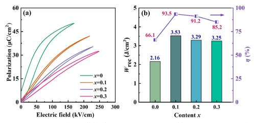
(a) Unipolar P-E loops at critical electric fields of (0.8 - x)BNT-BZT-xNN ceramics and (b)  $W_{rec}$  and  $\eta$  are calculated from (a).
