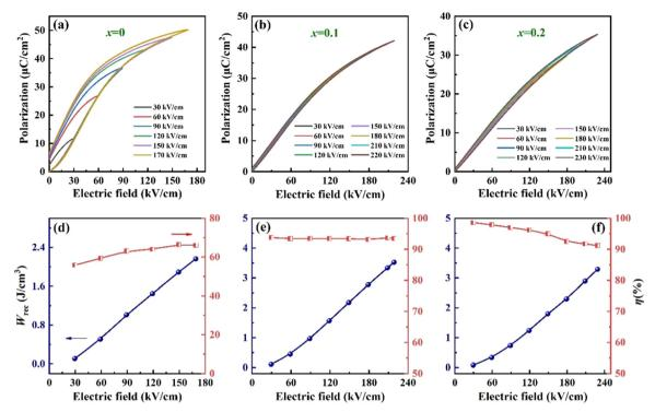
Fig. 7 (a)–(c) Unipolar P-E loops under different electric fields, and (d)–(f) electric-field dependence of  $W_{rec}$  and  $\eta$ .
