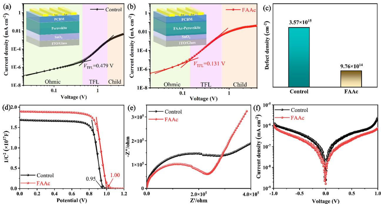
Fig. 4 (a) and (b) Dark  $J$ - $V$  curves of the devices with the structure of ITO/SnO<sub>2</sub>/control or FAAC-modified perovskite/PCBM/Au. (c) Statistics for defect density computed from the dark  $J$ - $V$  curves. (d) Mott-Schottky plots of control and FAAC-treated devices. (e) Nyquist plots and (f)  $J$ - $V$  curves under dark conditions of control and FAAC-treated devices.
