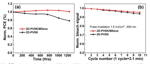
Fig. 6 (a) Stability of the PCE under open-air conditions and (b) photostability under fs pulse excitation for pristine and MXene-passivated PSC. The pump pulse was 1.5 mJ cm<sup>-2</sup> at 600 nm, and TA amplitude at 712 nm and fixed time delay at 6 ps after excitation (maximum of the bulk bleach signal) is taken to monitor the photodegradation
