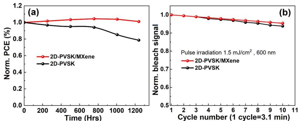
Fig. 6 (a) Stability of the PCE under open-air conditions and (b) photostability under fs pulse excitation for pristine and MXene-passivated PSC. The pump pulse was  $1.5 \text{ mJ cm}^{-2}$  at 600 nm, and TA amplitude at 712 nm and fixed time delay at 6 ps after excitation (maximum of the bulk bleach signal) is taken to monitor the photodegradation.
