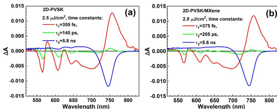
Fig. 7 Wavelength-dependant amplitudes of the indicated time constants from a 3-exponential global fit of TA data excited from HTL side at 475 nm with  $2.5 \text{ }\mu\text{J cm}^{-2}$  pump fluence for the cells: (a) without MXene and (b) with MXene.
