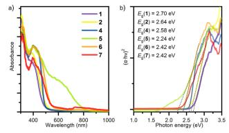
Fig. 5 (a) Kubelka-Munk diffuse reflectance absorption spectrum of compounds  $(NH_4)[VO_2(L^1)]$  (1),  $[VO(L^1)(OMe)(MeOH)]$  (2),  $[VO_2(HL^2)]$  (4)  $[VO(L^3)(OEt)(H_2O)]$  (5),  $[VO_2(HL^3)]_2 \cdot 2H_2O$  (6) and  $[VO(L^3)(OMe)(MeOH)]$ (7); and (b) direct optical transitions. Dashed lines indicate the band gap energies.
