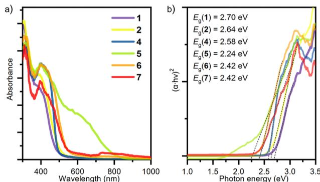
Fig. 5 (a) Kubelka–Munk diffuse reflectance absorption spectrum of compounds  $(\text{NH}_4)[\text{VO}_2(\text{L}^1)]$  (1),  $[\text{VO}(\text{L}^1)(\text{OMe})(\text{MeOH})]$  (2),  $[\text{VO}_2(\text{HL}^2)]$  (4),  $[\text{VO}(\text{L}^3)(\text{OEt})(\text{H}_2\text{O})]$  (5),  $[\text{VO}_2(\text{HL}^3)]_2 \cdot 2\text{H}_2\text{O}$  (6) and  $[\text{VO}(\text{L}^3)(\text{OMe})(\text{MeOH})]$  (7); and (b) direct optical transitions. Dashed lines indicate the band gap energies.
