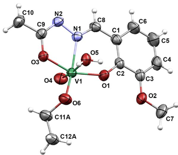
Fig. 2 Molecular structure of  $[\text{VO}(\text{L}^3)(\text{OEt})(\text{H}_2\text{O})]$  (5). The displacement ellipsoids are drawn at 30% probability level at 298 K. Hydrogen atoms are presented as spheres of arbitrary small radii.
