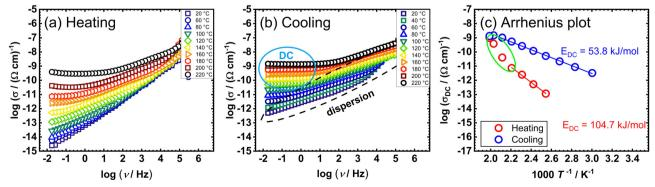
Fig. 7 Conductivity spectra for mononuclear ( $NH_4$ )[ $VO_2(L^1)$ ] sample (complex 1) in heating (a) and cooling (b) runs, and (c) temperature dependence of DC conductivity (log( $\sigma_{DC}$ ) vs. 1000/T) for both runs (red circle—heating, blue circle—cooling).
