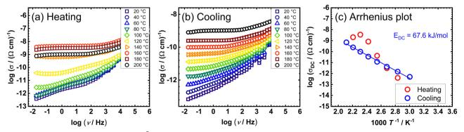
Fig. 9 Conductivity spectra for dinuclear  $[VO_2(L^3)]_2 \cdot 2H_2O$  sample (complex 6) in heating (a) and cooling (b) runs, and (c) temperature dependence of DC conductivity ( $log(\sigma_{DC})$  vs. 1000/T) for both runs (red circle – heating, blue circle – cooling)
