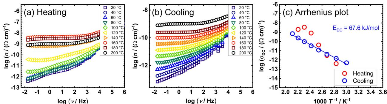
Fig. 9 Conductivity spectra for dinuclear  $[\text{VO}_2(\text{L}^3)]_2 \cdot 2\text{H}_2\text{O}$  sample (complex **6**) in heating (a) and cooling (b) runs, and (c) temperature dependence of DC conductivity ( $\log(\sigma_{\text{DC}})$  vs.  $1000/T$ ) for both runs (red circle – heating, blue circle – cooling).
