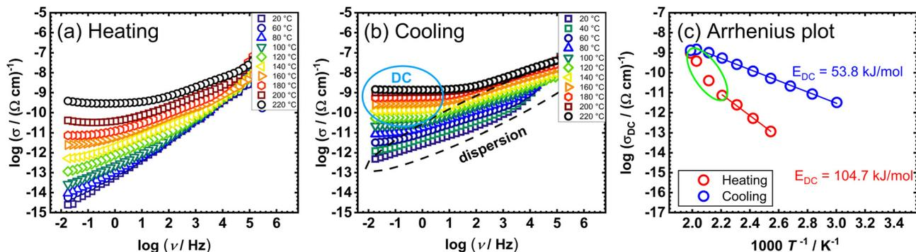
Fig. 7 Conductivity spectra for mononuclear  $(\text{NH}_4)[\text{VO}_2(\text{L}^1)]$  sample (complex 1) in heating (a) and cooling (b) runs, and (c) temperature dependence of DC conductivity ( $\log(\sigma_{\text{DC}})$  vs.  $1000/T$ ) for both runs (red circle—heating, blue circle—cooling).
