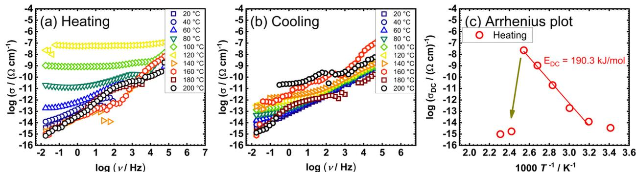
Fig. 8 Conductivity spectra for mononuclear  $[\text{VO}(\text{L}^3)(\text{OEt})(\text{H}_2\text{O})]$  sample (complex **5**) in heating (a) and cooling (b) runs, and (c) temperature dependence of DC conductivity ( $\log(\sigma_{\text{DC}})$  vs.  $1000/T$ ) for both runs (red circle – heating, blue circle – cooling).
