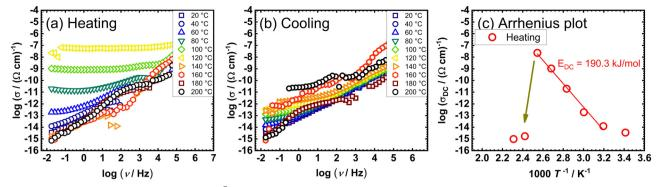
Fig. 8 Conductivity spectra for mononuclear [VO(L<sup>3</sup>)(OEt)(H<sub>2</sub>O)] sample (complex 5) in heating (a) and cooling (b) runs, and (c) temperature dependence of DC conductivity ( $log(\sigma_{DC})$  vs. 1000/T) for both runs (red circle – heating, blue circle – cooling).
