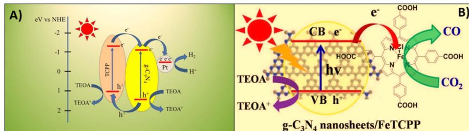
Fig. 36 (A) Suggested mechanism for photocatalytic  $\text{H}_2$  evolution over TCPP/ $g\text{-C}_3\text{N}_4$ /Pt under visible light irradiation ( $\lambda > 380$  nm). Reproduced from ref. 162. Copyright 2017 Elsevier. (B) Structure of the  $g\text{-C}_3\text{N}_4$ /FeTCPP heterogeneous catalyst. Adapted from ref. 171, Copyright 2018 Elsevier.
