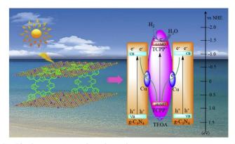
Fig. 38 Scheme of the TCPP-Cu-g-C<sub>3</sub>N<sub>4</sub> composite and illustration of the separation and transfer of photo-produced charges promoted by this photocatalyst. Reproduced from ref. 164. Copyright 2019 Elsevier
