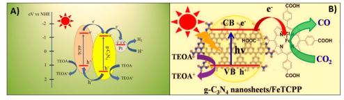
Fig. 36 (A) Suggested mechanism for photocatalytic  $H_2$  evolution over TCPP/g- $C_3N_4$ /Pt under visible light irradiation ( $\lambda > 380$  nm). Reproduced from ref. 162. Copyright 2017 Elsevier. (B) Structure of the g-C<sub>3</sub>N<sub>4</sub>/FeTCPP heterogeneous catalyst. Adapted from ref. 171, Copyright 2018 Elsevier.
