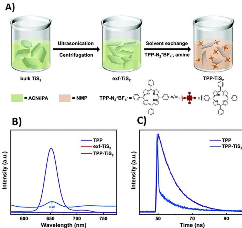
Fig. 42 (A) Diagram illustrating the preparation process of TPP-modified  $\text{TiS}_2$  sheets from bulk  $\text{TiS}_2$ , (B) photoluminescence spectra of free TPP, exfoliated (exf)- $\text{TiS}_2$ , and TPP- $\text{TiS}_2$  hybrid, and (C) fluorescence decay profiles (excitation at 405 nm) of free TPP and TPP- $\text{TiS}_2$ . Reproduced from ref. 182.
