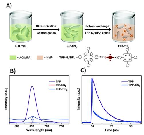
Fig. 42 (A) Diagram illustrating the preparation process of TPP-modified TiS2 sheets from bulk TiS2, (B) photoluminescence spectra of free TPP, exfoliated (exf)-TiS2, and TPP-TiS2 hybrid, and (C) fluorescence decay profiles (excitation at 405 nm) of free TPP and TPP-TiS2. Reproduced from ref. 182.
