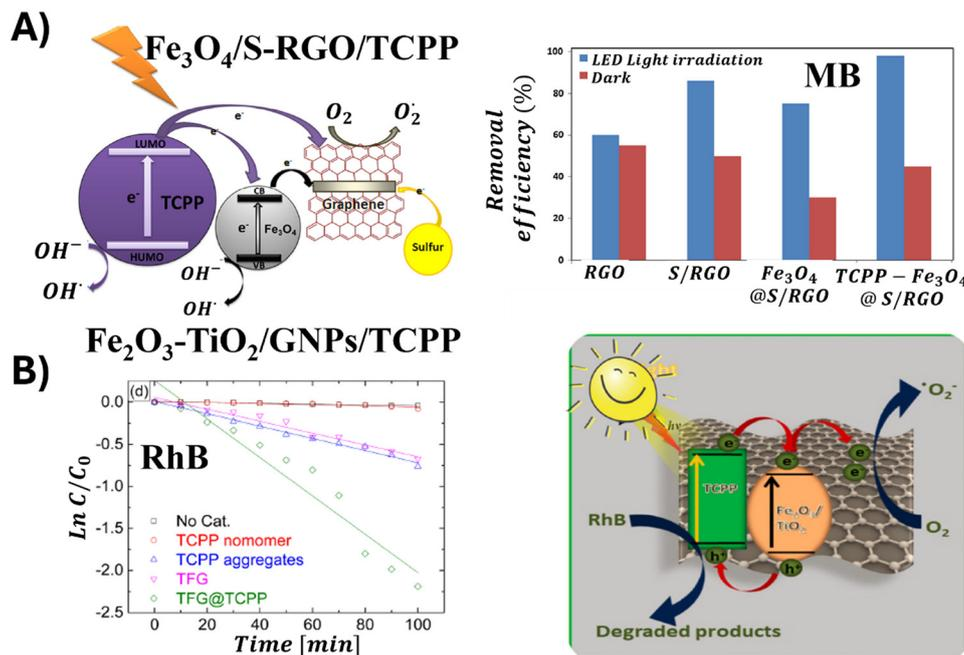
Fig. 33 (A) Mechanism of MB photodegradation catalyzed by  $\text{Fe}_3\text{O}_4/\text{S-RGO}/\text{TCPP}$ . Adapted with permission from ref. 156. Copyright 2015, Springer Science Business Media Dordrecht. (B) Mechanism of RhB photodegradation catalyzed by  $\text{Fe}_2\text{O}_3\text{-TiO}_2/\text{GNPs}/\text{TCPP}$ . Adapted with permission from ref. 155. Copyright 2021 Elsevier Ltd.
