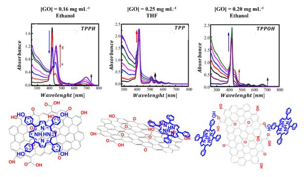
UV-vis absorption spectra and structural schemes of TPPH/GO, TPP/GO, and TPPOH/GO. Adapted with permission from ref. 95. Copyright 2015 Elsevier.
