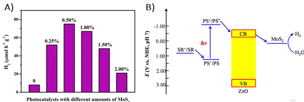
**Fig. 40** (A) Photocatalytic H<sub>2</sub> evolution over ZnTCPP/MoS<sub>2</sub>/ZnO photocatalysts with different co-catalyst loadings in a 0.2 M TEOA aqueous solution under visible light irradiation ( $\lambda > 420$  nm). (B) Suggested mechanism for visible-light-induced hydrogen production using ZnTCPP/MoS<sub>2</sub>/ZnO, photosensitizer (PS): ZnTCPP, sacrificial reagent (SR): TEOA. Reproduced with permission from ref. 176. Copyright 2015 Elsevier.
