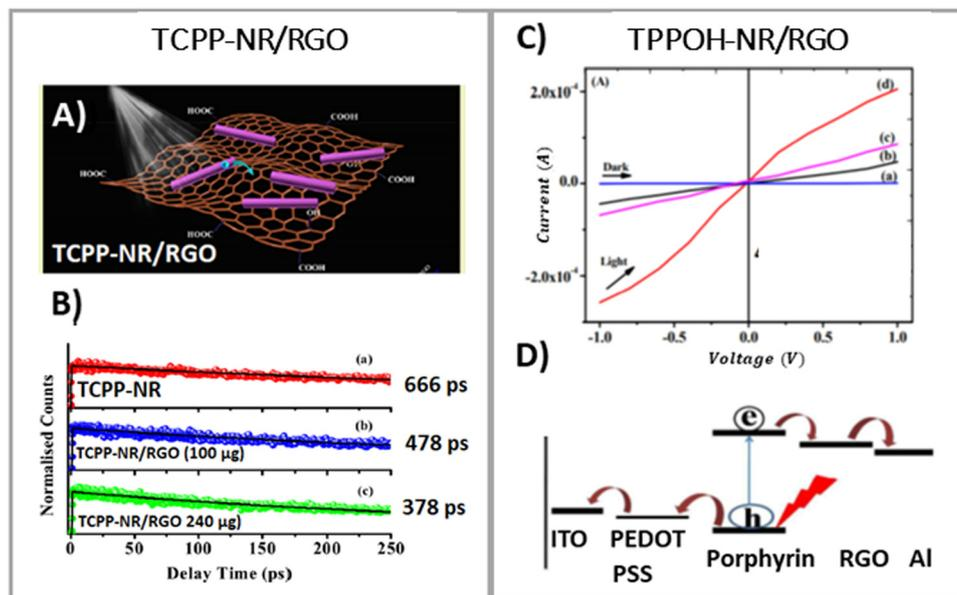
Fig. 21 (A) Schematic of the TCPP-NR/RGO system exposed to light irradiation. (B) Comparative fluorescence decays of free TCPP-NR and TCPP-NR/RGO composites. Adapted from ref. 118. Copyright 2016, American Chemical Society. (C) Photocurrent generation with pure porphyrin and TPPOH-NR/RGO hybrid as active materials on the photoanode. (D) Schematic energy-level diagram and charge separation path in the tested device. Adapted from ref. 116 with permission from the Royal Society of Chemistry.
