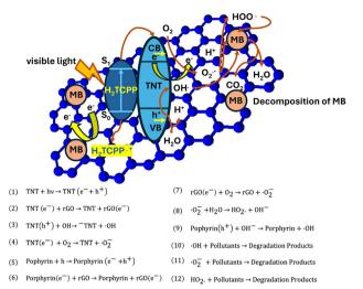
Fig. 31 Diagram depicting the photocatalytic activity of the TCPP/RGO/ (TiO<sub>2</sub> nanotubes = TNT) during the degradation of MB pollutants, including the light-initiated reactions within this photocatalytic system. Adapted with permission from ref. 150. Copyright 2016 Hydrogen Energy Publications LLC.
