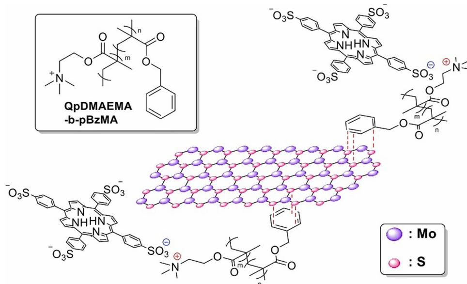
Fig. 41 Illustrative structure of the MoS<sub>2</sub>/QpDMAEMA-*b*-pBzMA/TPPS nanohybrid. Reproduced with permission from ref. 177. Copyright 2024 Elsevier Inc.
