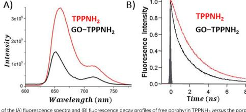
Fig. 15 Comparison of the (A) fluorescence spectra and (B) fluorescence decay profiles of free porphyrin TPPNH<sub>2</sub> versus the porphyrin covalently bound to GO. Adapted with permission from ref. 59. Copyright 2011, Royal Society of Chemistry.
