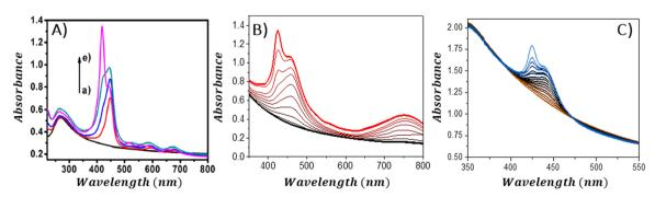
Fig. 11 Absorption spectra obtained during the titration of the GBM solution (constant concentration) with the increase in the amount of porphyrin: (A) TPPH added to RGO; (B) TAPP to GO and (C) ZnTPPH to GO. Reproduced from ref. 85, 96 and 97. Copyright 2013, American Chemical Society.
