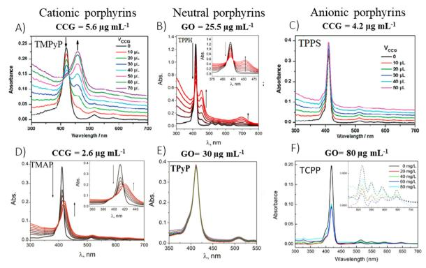
Fig. 7 Titration-induced changes in the absorption spectra for various porphyrin/GBM: (A) TMPyP with CCG, (B) TPPH with GO, (C) TPPS with CCG, (D) TMAP with CCG, (E) TPyP with GO and (F) TCPP with GO. The concentrations listed above each panel indicate the final GBM concentration achieved upon completion of the porphyrin solution titration. Adapted from ref. 72, 80-82. Copyright 2019 American Chemical Society, Copyright 2009 American Chemical Society, Copyright 2019 John Wiley and Sons.
