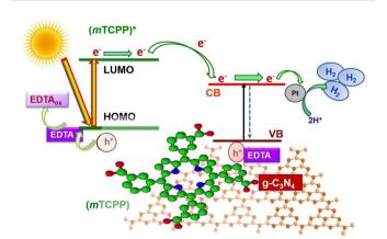
Fig. 37 Mechanism of photocatalytic hydrogen production from water over g-C<sub>3</sub>N<sub>4</sub> sensitized with m-TCPP porphyrin. Reproduced from ref. 163. Copyright 2018 Elsevier.
