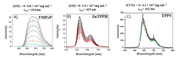
Fig. 12 Quenching of the fluorescence of (A) TMPyP in the presence of GO, (B) ZnTPPH in the presence of GO and (C) TPPS in the presence of CCG. Adapted with permission from ref. 73, 80 and 84. Copyright 2019 Wiley-VCH Verlag GmbH & Co. KGaA, Weinheim and Copyright 2009 American Chemical Society.
