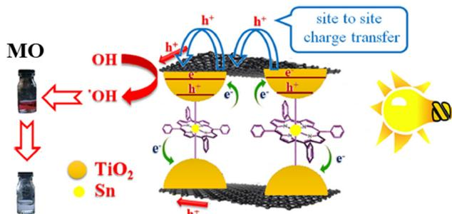
**Fig. 32** Diagram depicting the charge transfer process in the prepared SnTCPP/graphene/ $\text{TiO}_2$  hybrid exposed to visible light irradiation. Adapted with permission from ref. 152. Copyright © 2015 Elsevier Inc.
