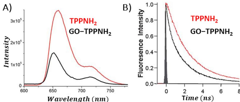
Fig. 15 Comparison of the (A) fluorescence spectra and (B) fluorescence decay profiles of free porphyrin TPPNH<sub>2</sub> versus the porphyrin covalently bound to GO. Adapted with permission from ref. 59. Copyright 2011, Royal Society of Chemistry.
