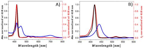
Fig. 14 (A) Normalized fluorescence excitation spectrum of the mixture of TPPH and GO (red), absorption spectrum of this mixture (blue) and normalized absorption spectrum of TPPH in the absence of GO (black). (B) Normalized fluorescence excitation spectrum of the mixture of TPPH and RGO (red), absorption spectrum of this mixture (blue) and normalized absorption spectrum of TPPH in the absence of RGO (black). Reproduced from ref 85
