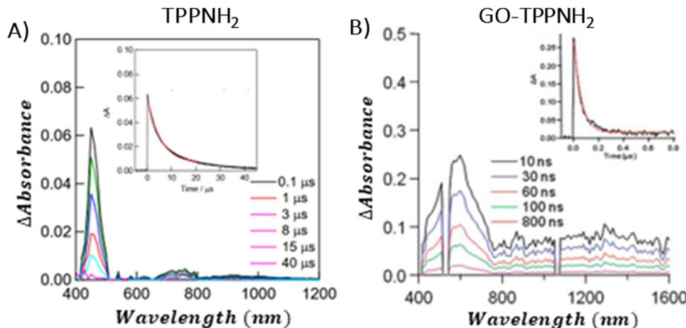
Fig. 19 Nanosecond TAS for: (A) free TPPNH<sub>2</sub> (inset: TA decay at 450 nm) and (B) covalent hybrid GO-TPPNH<sub>2</sub> (inset: TA decay at 610 nm). Adapted from ref. 116. Copyright 2011, Royal Society of Chemistry.
