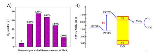
Fig. 40 (A) Photocatalytic H<sub>2</sub> evolution over ZnTCPP/MoS<sub>2</sub>/ZnO photocatalysts with different co-catalyst loadings in a 0.2 M TEOA aqueous solution under visible light irradiation ( $\lambda > 420$  nm). (B) Suggested mechanism for visible-light-induced hydrogen production using ZnTCPP/MoS<sub>2</sub>/ZnO, photosensitizer (PS): ZnTCPP, sacrificial reagent (SR): TEOA. Reproduced with permission from ref. 176. Copyright 2015 Elsevier.
