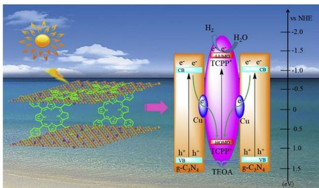
Fig. 38 Scheme of the TCPP–Cu– $g\text{-C}_3\text{N}_4$  composite and illustration of the separation and transfer of photo-produced charges promoted by this photocatalyst. Reproduced from ref. 164. Copyright 2019 Elsevier.
