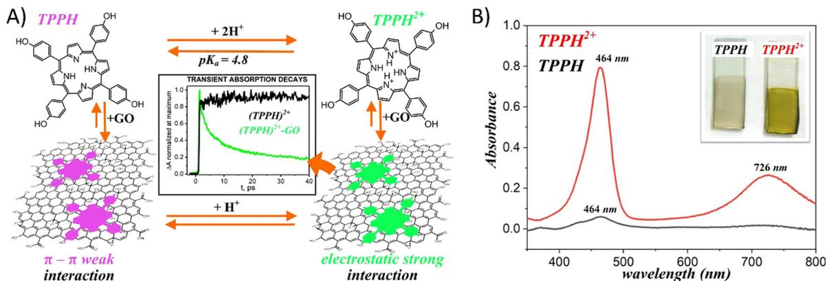
Fig. 9 (A) Schematic of the pH influence on the interaction of TPPH with GO. (B) Comparison of the adsorption of porphyrins (TPPH (black) and cationic TPPH<sup>2+</sup> (red)) from solutions on GO films monitored by UV-vis spectroscopy. Adapted with permission from ref. 72. Copyright 2019 American Chemical Society.
