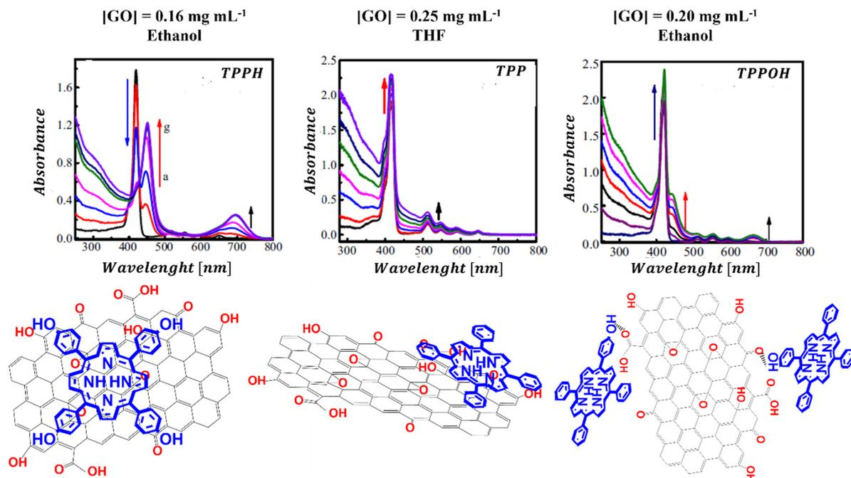
Fig. 10 UV-vis absorption spectra and structural schemes of TPPH/GO, TPP/GO, and TPPOH/GO. Adapted with permission from ref. 95. Copyright 2015 Elsevier.
