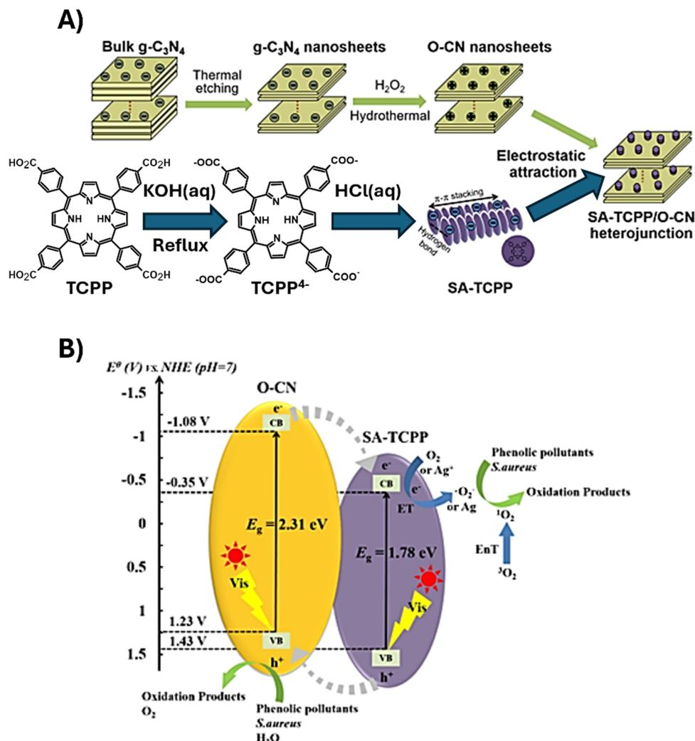
**Fig. 39** (A) Synthesis of g-C<sub>3</sub>N<sub>4</sub>-O, SA-TCPP and SA-TCPP/g-C<sub>3</sub>N<sub>4</sub>-O heterojunctions and (B) schematic representation of the proposed carrier separation and photocatalytic processes under visible light irradiation in the SA-TCPP/g-C<sub>3</sub>N<sub>4</sub>-O heterojunction catalyst. Reproduced from ref. 168 Copyright 2021 Elsevier.
