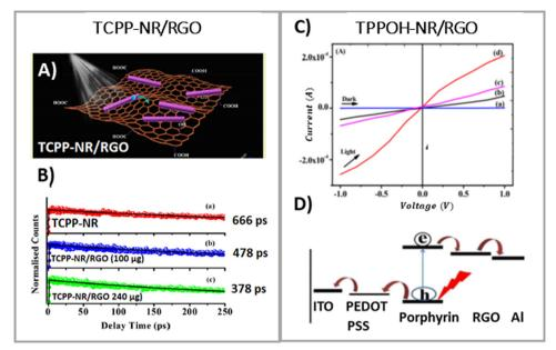
Fig. 21 (A) Schematic of the TCPP-NR/RGO system exposed to light irradiation. (B) Comparative fluorescence decays of free TCPP-NR and TCPP-NR/ RGO composites. Adapted from ref. 118. Copyright 2016, American Chemical Society. (C) Photocurrent generation with pure porphyrin and TPPOH-NR/ RGO hybrid as active materials on the photoanode. (D) Schematic energy-level diagram and charge separation path in the tested device. Adapted from ref. 116 with permission from the Royal Society of Chemistry.
