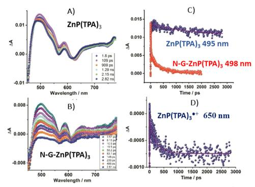
Fig. 20 Femtosecond TAS at indicated delay times for (A) ZnP(TPA)<sub>3</sub> control and (B) its hybrid with N-G, (C) TA decays for <sup>1</sup>ZnP(TPA)<sub>3</sub>\*: control at 495 nm (free porphyrin) and hybrid at 498 nm (porphyrin bound to N-G), (D) time profile for the 650 nm peak corresponding to ZnP(TPA)3. Adapted from ref. 113
