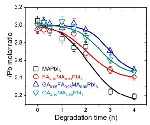
Fig. 3 Surface EDS iodine-to-lead molar ratio quantification as a function of time for samples treated at 200 °C. Lines were added as guides for the
