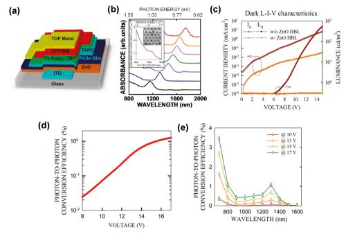
Fig. 11 (a) Schematic diagram of device structure. (b) Absorption spectra of various QDs. (c) Dark L-I-V characteristic curves. (d) and (e) Up-conversion efficiency.<sup>37</sup> Copyright 2011, American Chemical Society.
