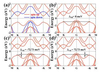
Fig. 4 (a) The band structure of the  $SVSiN_2$  monolayer without SOC. (b)-(d) The band structure of the SVSiN<sub>2</sub> monolayer with SOC, where (b)-(d) represent the magnetic moment of V ions in the +x, +z, and -z directions, respectively
