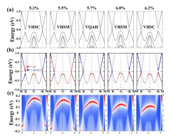
Fig. 7 The (a) band structure of the SVSiN<sub>2</sub> monolayer containing SOC under biaxial strain. The corresponding (b) orbital-resolved band structure and (c) edge state of the SVSiN<sub>2</sub> monolayer under biaxial strain.
