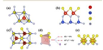
Fig. 1 Top- (a) and side-views (b) of the primitive structure of the SVSiN<sub>2</sub> monolayer. (c) The top view of a rectangular supercell for magnetic ground state calculations. For the AFM configuration, the spin directions are marked with black arrows. (d) A schematic diagram of the d-orbital energy levels of the V ion in a trigonal prismatic crystal field, and (e) shows the spin density distribution of the SVSiN2 monolayer.
