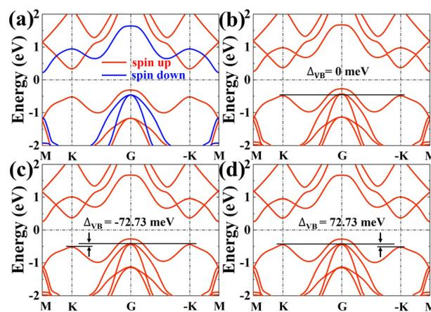
Fig. 4 (a) The band structure of the SVSiN<sub>2</sub> monolayer without SOC. (b)–(d) The band structure of the SVSiN<sub>2</sub> monolayer with SOC, where (b)–(d) represent the magnetic moment of V ions in the  $+x$ ,  $+z$ , and  $-z$  directions, respectively.
