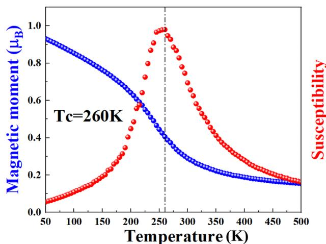
Fig. 3 The Curie temperature of the SVSiN<sub>2</sub> monolayer based on Monte Carlo simulations.
