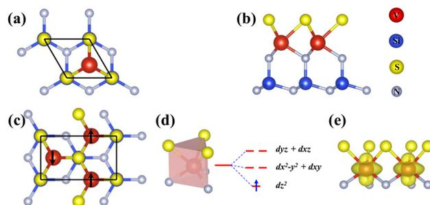
Fig. 1 Top- (a) and side-views (b) of the primitive structure of the  $\text{SVSiN}_2$  monolayer. (c) The top view of a rectangular supercell for magnetic ground state calculations. For the AFM configuration, the spin directions are marked with black arrows. (d) A schematic diagram of the d-orbital energy levels of the V ion in a trigonal prismatic crystal field, and (e) shows the spin density distribution of the  $\text{SVSiN}_2$  monolayer.
