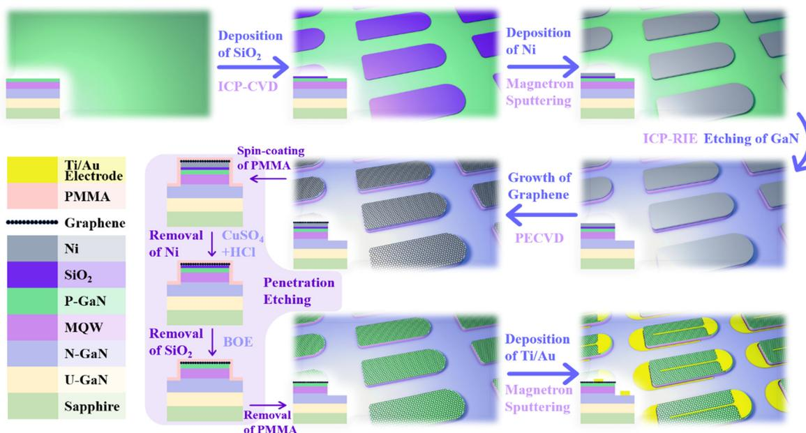
**Fig. 1** Schematic diagram of the process flow and chip structures of LEDs with transfer-free patterned graphene as transparent electrodes. Three-dimensional diagrams and cross-sectional diagrams are presented for clearer illustration. Abbreviations: ICP, inductively coupled plasma; CVD, chemical vapor deposition; RIE, reactive ion etching; PECVD, plasma enhanced chemical vapor deposition; BOE, buffered oxide etching; MQW, multiple quantum well.
