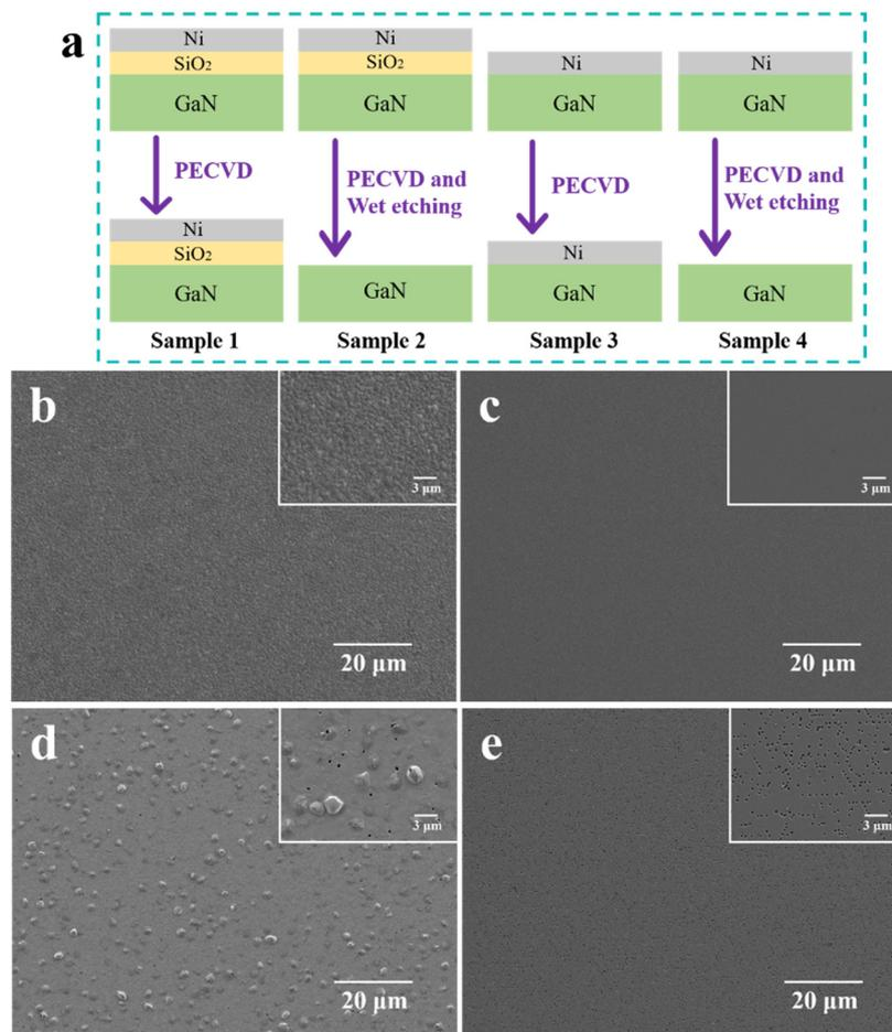
Fig. 5 Four samples were prepared to explore the effect of 650 °C temperature on Ni and GaN as well as the isolation effect of SiO<sub>2</sub>. (a) The structural diagram and processing method of the samples. The thickness of the Ni layer is 250 nm, and the thickness of the SiO<sub>2</sub> layer is 100 nm. (b)–(e) SEM images (SE2 mode) of samples 1–4 in sequence.
