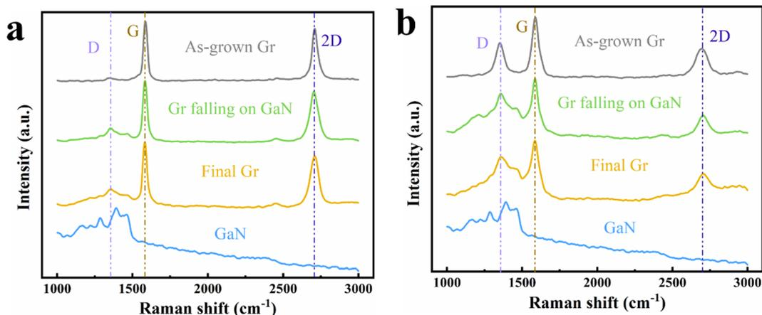
Fig. 3 Raman spectra of graphene grown with (a) and without (b) isolation layer at different experimental stages. As-grown Gr: graphene grown on the surface of Ni; Gr falling on GaN: graphene that “falls” on the surface of GaN after penetration etching; final graphene: after the fabrication of electrodes, the final graphene on the LED.
