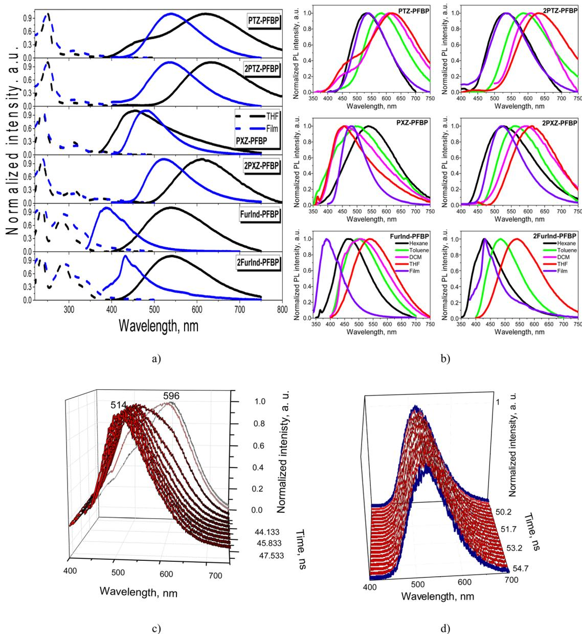
Fig. 5 Absorption and PL spectra (a) of dilute THF solutions and solid films of **PFBP** derivatives and PL spectra (b) of dilute solutions and solid films of the compounds. Normalized sliced PL spectra of the THF solution (c) and neat film (d) of **PTZ-PFBP** recorded at different times after excitation.
