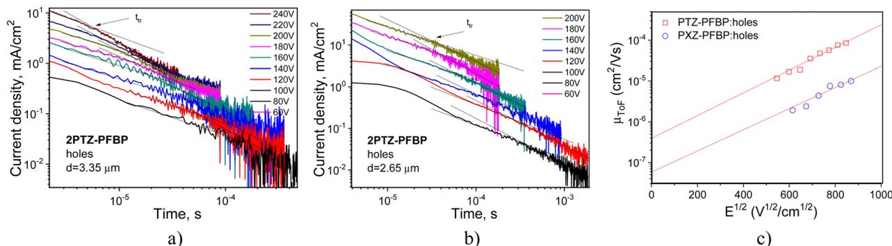
Fig. 9 TOF current transients for holes (a) and (b) observed for vacuum-deposited films of compounds **2PTZ-PFBP** and **2PXZ-PFBP** at different electric fields. Electric field dependence of hole mobilities presented according the Poole-Frenkel law ( $\mu = \mu_0 \exp \beta E^{1/2}$ ) and the corresponding fitting lines (c).
