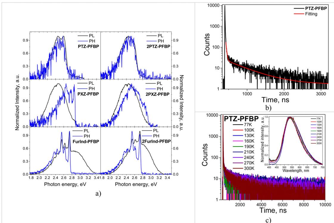
Fig. 7 PL and Ph spectra (a) of the solutions of the derivatives of **PFBP** in THF recorded at 77 K; PL decay curves of the film of **PTZ-PFBP** recorded at room temperature (b) and at different (c) temperatures ( $\lambda_{em} = 534$  nm).
