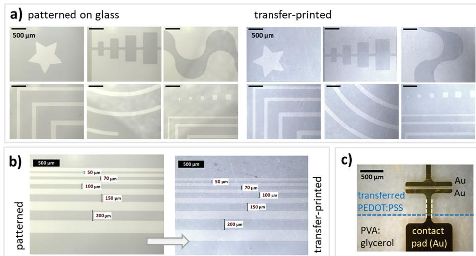
Fig. 3 (a) Selection of microscope images of the  $O_2$ -patterned PEDOT:PSS thin films on glass (left) and transfer-printed on to PVA:glycerol (25 wt%) substrates (right). (b) Patterned and transfer-printed stripes (minimal width: 50  $\mu\text{m}$ ). (c) Patterned PEDOT:PSS on PVA:glycerol substrates with top gold contacts (thermally evaporated in vacuum) for device applications. The length of each scale bar is 500  $\mu\text{m}$ .
