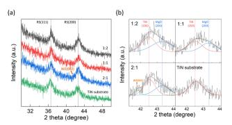
Fig. 4 (a) Grazing incidence X-ray diffraction (GIXRD) spectra of BMO samples following post-deposition annealing (PDA) at 500 °C, compared with a bare TiN substrate. (b) An expanded view of the GIXRD spectra in the 2 theta range of 41-44°, featuring background subtraction and peak deconvolution for detailed analysis
