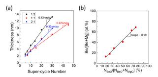
Fig. 2 (a) Relationship between the number of super-cycles and film thickness (growth per cycle, GPC) for various sub-cycle ratios. (b) Correlation between sub-cycle ratio and atomic ratio, estimated by AES (see Fig. S1, ESI† for details).
