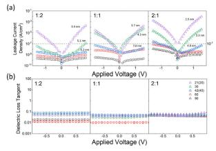
Fig. 7 Electrical characterization of BMO-based metal-insulator-metal (MIM) devices, showing (a) current density-voltage (J-V) curves, and (b) dielectric loss tangent plots. These measurements are for devices with various total ALD cycle counts: 90, 60, 42 (40 for the 1:1 ratio), 30, and 21 (20 for the 1:1 ratio). The thicknesses of the three thinnest BMO films in each case are noted in (a)
