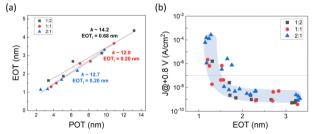
**Fig. 6** Plots illustrating the electrical characteristics of BMO-based metal-insulator-metal (MIM) devices: (a) equivalent oxide thickness (EOT) *versus* physical oxide thickness (POT) plot. (b) Leakage current density (*J*) *versus* EOT plot.
