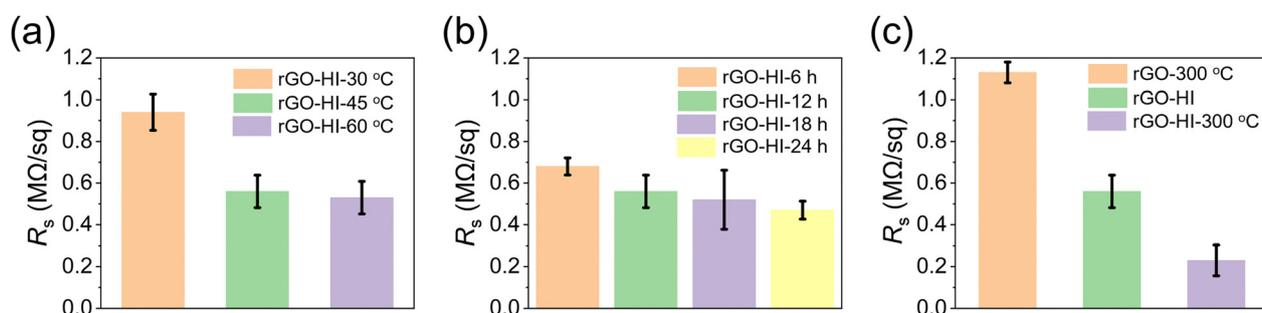
Fig. 3 (a)  $R_s$  of the rGO films reduced by HI vapor at 30, 45 and 60 °C for 12 h, respectively. (b)  $R_s$  of the rGO films reduced by HI vapor at 45 °C for 6, 12, 18, and 24 h, respectively. (c)  $R_s$  of the rGO-300 °C, rGO-HI, and rGO-HI-300 °C films, respectively.
