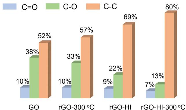
Fig. 4 The intensity ratios of C=O, C-O, and C-C peaks, obtained from the C1s XPS spectra of GO, rGO-300 °C, rGO-HI, and rGO-HI-300 °C, respectively.
