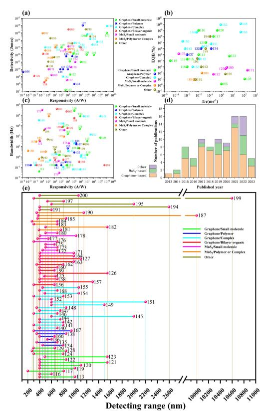
Fig. 17 (a) Responsivity and detectivity of 2D/organic heterojunction photodetectors. (b) EQE and 1/τ of 2D/organic heterojunction photodetectors. (c) Bandwidth and responsivity of 2D/organic heterojunction photodetectors. (d) The number of publications of 2D/organic heterojunction photodetectors. (e) The detection range of 2D/organic heterojunction photodetectors. Note: bandwidth =  $1/(2\pi\tau)$ .
