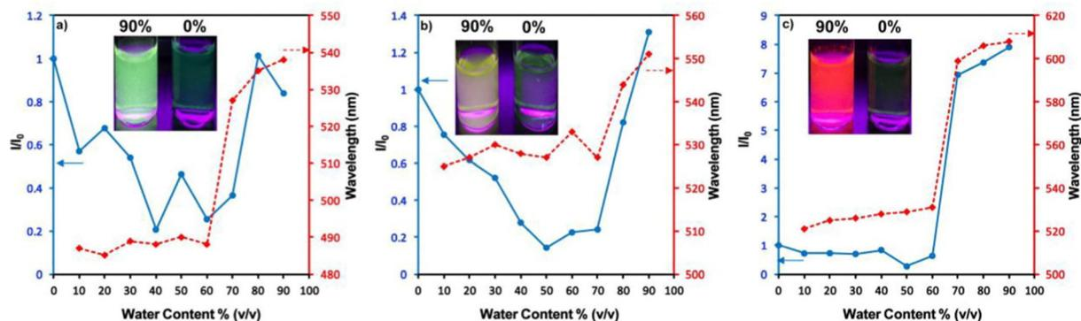
Fig. 19 Changes in the PL intensity and  $k_{\text{max}}$  in THF–water mixtures with  $f_w = 10$ –90%: (a) compound **24**, (b) compound **25** and (c) compound **26**. Inset: Fluorescence images of the luminogens in THF–water mixtures at  $f_w = 90\%$  and  $f_w = 0\%$  under illumination with a 365 nm UV lamp. Reproduced with permission from ref. 87. Copyright 2021 Elsevier.
