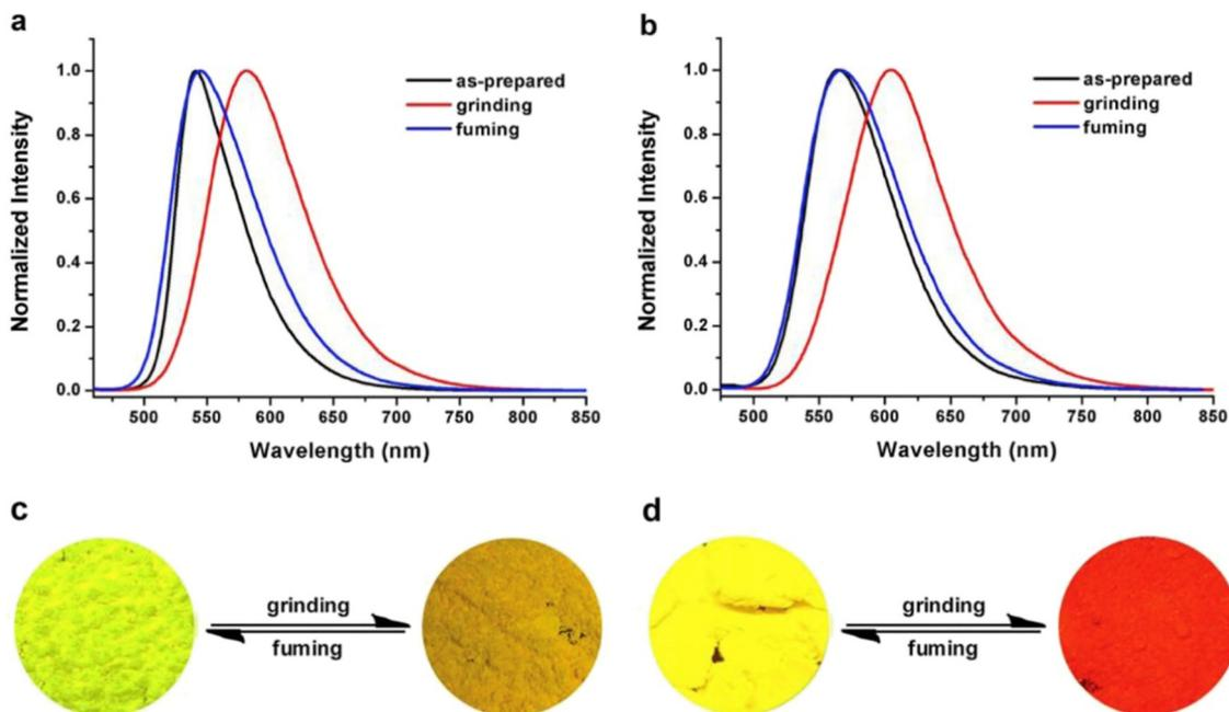
Fig. 9 Normalized fluorescence spectra of compound **12** (a) and compound **13** (b) excited at 450 nm in different solid-state conditions: as-prepared, ground and fumed. Photographs of the color changes of compound **12** (c) and compound **13** (d) under grinding and fuming. Reproduced with permission from ref. 80. Copyright 2018 Elsevier.
