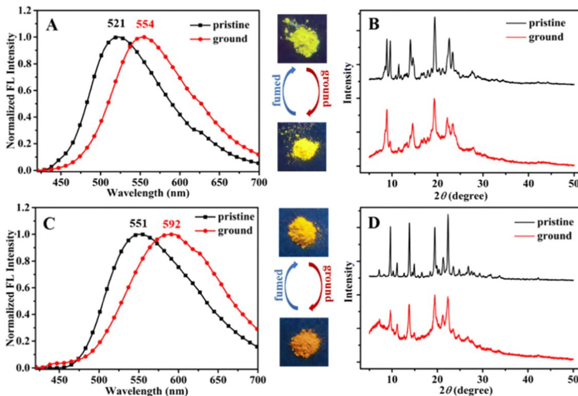
Fig. 7 Fluorescence spectra (A) and (C) and powder XRD patterns (B) and (D) of compounds **9** and **11**, respectively. Inset: Fluorescence images under 365 nm UV light. Reproduced with permission from ref. 75. Copyright 2022 Royal Society of Chemistry.
