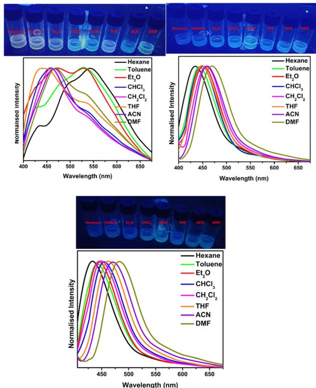
Fig. 31 The FL spectra of compound **43a** (top left), **43b** (top right) and **43c** (bottom) at various solvents; inset: digital photos taken under 365 nm UV light. Reproduced with permission from ref. 42. Copyright 2023 Royal Society of Chemistry.
