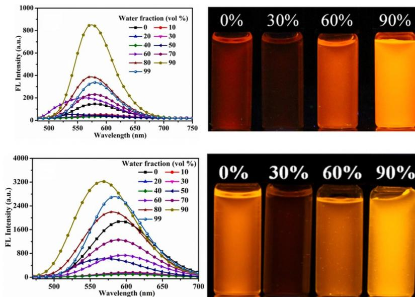
Fig. 5 Fluorescence spectra of compounds **4** and **6** with different fractions of water (left), and the corresponding images under 365-nm UV light (right). Reproduced with permission from ref. 75. Copyright 2021 Elsevier.
