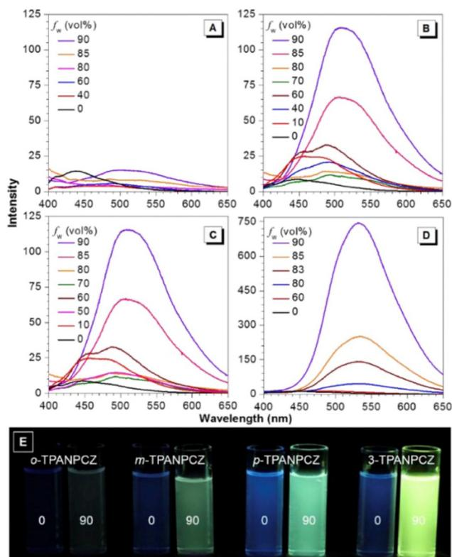
Fig. 27 Emission spectra of (A) compound **38**, (B) compound **39**, (C) compound **40** and (D) compound **41** in THF and THF/water mixtures with varying  $f_w$  values. (E) Photographs of the luminogens in THF and a 10/90 THF/water mixture taken under 365 nm UV illumination. Reproduced with permission from ref. 92. Copyright 2018 Elsevier.
