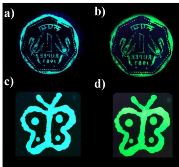
Fig. 16 (a) Data encryption of Indian 1-rupee coin on an aluminium foil using compound **21b** immersed in chloroform and dried. (b) The sealed coin after fuming with DMF. (c) Butterfly pattern drawn on a filter paper using chloroform solution of compound **21b** and dried. (d) The butterfly pattern after fuming with DMF. Reproduced with permission from ref. 85. Copyright 2023 Elsevier.
