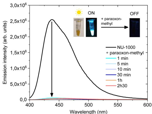
Fig. 6 NU-1000 emission spectra at  $\lambda_{\text{ex}} = 385$  nm recorded at different times during the degradation of paraoxon-methyl (1 mL of 1.3 mM NU-1000, 4  $\mu\text{L}$  of paraoxon-methyl, 500 $\times$  dilution prior to analysis).
