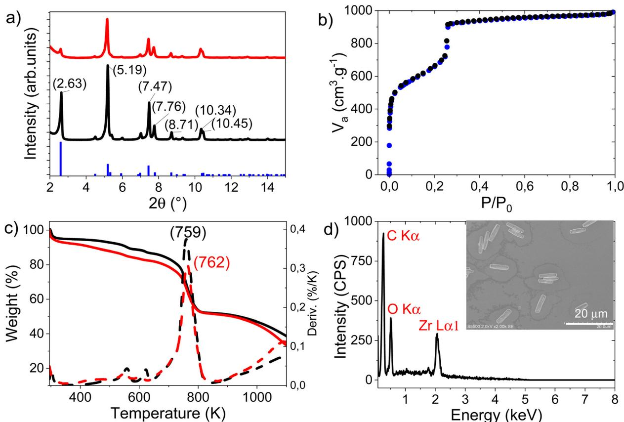
Fig. 1 (a) PXRD patterns of activated NU-1000 (black) and NU-1000/NEM (red) compared with the simulated reference pattern for NU-1000 (blue). (b)  $\text{N}_2$  adsorption (blue) and desorption (black) isotherms of as-synthesized NU-1000. (c) TGA traces of NU-1000, as-synthesized (black) or after contact with NEM buffer (NU-1000/NEM, red). (d) EDX spectrum of NU-1000/NEM with (inset) the SEM image of a NU-1000/NEM suspension.
