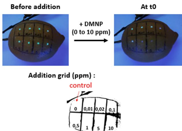
Fig. 9 Photographs under UV light (312 nm) of an organic lemon with a drop-cast film of 0.09 mM NU-1000/NEM and drops of paraoxon-methyl arranged in a grid.
