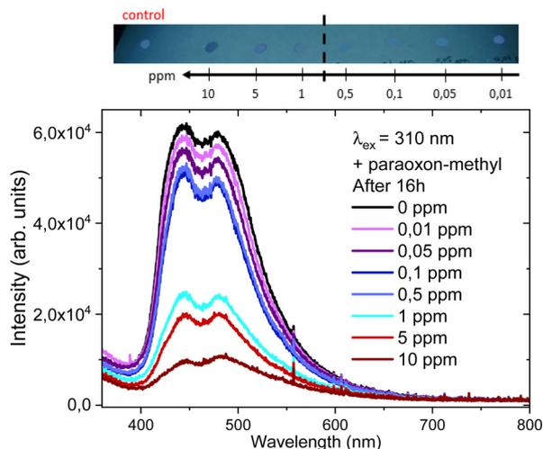
Fig. 8 NU-1000 emission intensity on cotton paper at different paraoxon-methyl concentrations (top) and measurements after 16 h using a portable spectrometer at  $\lambda_{\text{ex}} = 310$  nm (bottom).
