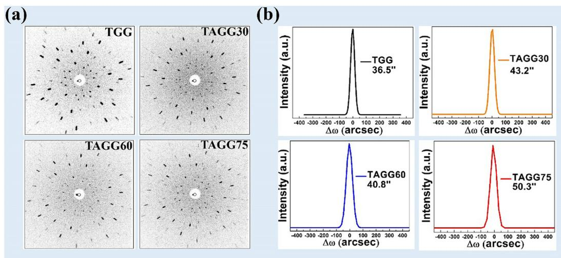
Fig. 3 Crystalline quality of as-grown TAGG crystals: (a) Laue back-reflection patterns. (b) Rocking curves.
