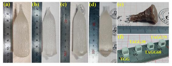
Fig. 1 Photographs of as-grown TAGG single crystals: (a) TGG, (b) TAGG30, (c) TAGG60, (d) TAGG75, and (e) TAGG90. (f) Polished crystal cubes.
