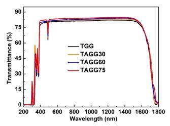
Transmittance of TAGG crystals
