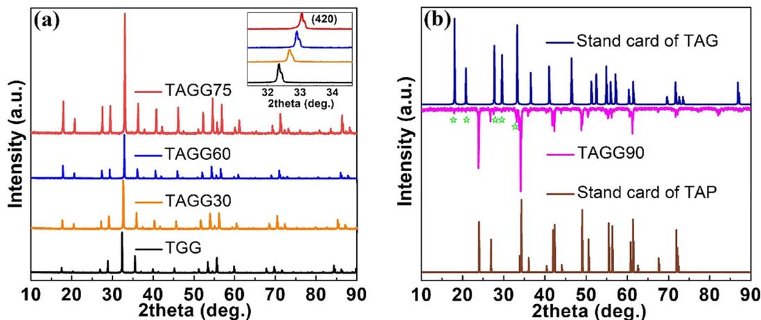
Fig. 2 (a) Powder XRD patterns of TAGG ( $x \leq 0.75$ ) crystals. The inset shows the right shift of the enlarged (420) diffraction peaks. (b) XRD patterns of TAGG90 as well as TAG and TAP for comparison.
