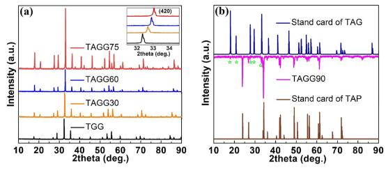
Fig. 2 (a) Powder XRD patterns of TAGG ( $x \le 0.75$ ) crystals. The inset shows the right shift of the enlarged (420) diffraction peaks. (b) XRD patterns of TAGG90 as well as TAG and TAP for comparison.
