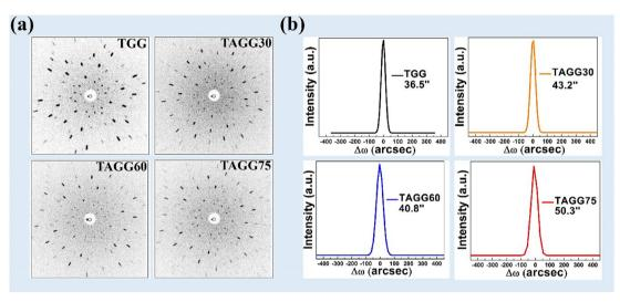
Fig. 3 Crystalline quality of as-grown TAGG crystals: (a) Laue back-reflection patterns. (b) Rocking curves.
