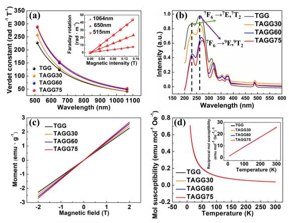
Fig. 6 (a) Verdet constant of TAGG crystals at the wavelengths of 532, 650, and 1064 nm. The inset shows the Faraday rotation angles of the TAGG75 crystal as a function of magnetic intensity and wavelength. (b) Diffuse reflection spectra of TAGG crystals. (c) The moment in the range of -2 T to 2 T at room temperature. (d) Temperature dependence of the mol susceptibility. The inset shows the reciprocal mol susceptibility versus temperature (H = 2 T).
