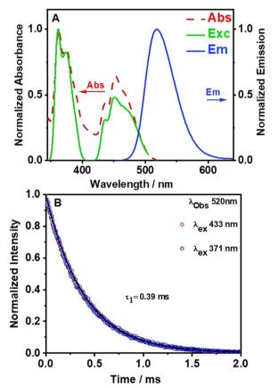
Fig. 3 (A) Normalized to the maximum intensity of reflectance (converted to the K-M function), excitation (observation at 520 nm), and emission (excitation at 365 nm) spectra of the (TPA)<sub>2</sub>MnBr<sub>4</sub> as-synthesized powder. (B) Emission decays of the (TPA)<sub>2</sub>MnBr<sub>4</sub> as-synthesized powder following excitation at 371 nm (blue circles) and 433 nm (red circles). The solid lines represent the best monoexponential fit
