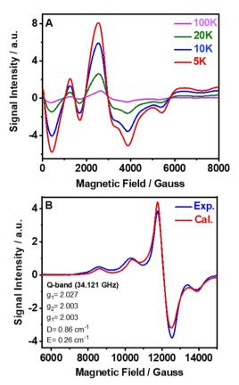
Fig. 2 (A) Variation of the X-band electron-spin paramagnetic resonance (EPR) spectra of (TPA)<sub>2</sub>MnBr<sub>4</sub> with temperature from 5 to 100 K. (B) Experimental and calculated Q-band room temperature spectra (see the text for details of the fit).
