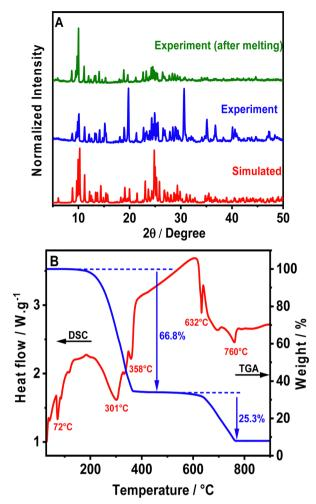
Fig. 1 (A) PXRD patterns of the powder sample of  $(TPA)_2MnBr_4$ , before and after melting, as well as the simulated PXRD pattern from SCXRD. (B) TGA-DSC curves of  $(TPA)_2MnBr_4$ .
