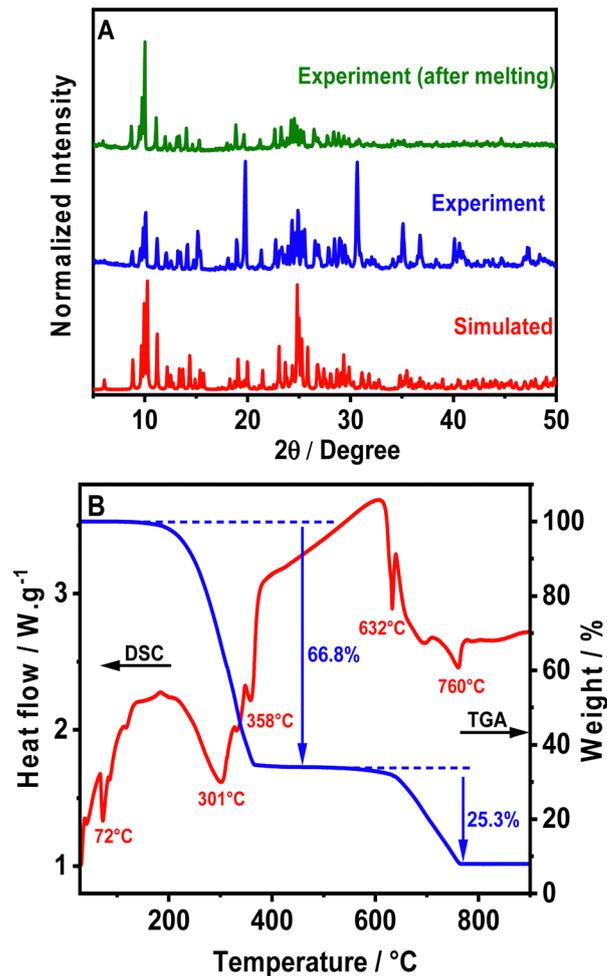
Fig. 1 (A) PXRD patterns of the powder sample of (TPA)<sub>2</sub>MnBr<sub>4</sub>, before and after melting, as well as the simulated PXRD pattern from SCXRD. (B) TGA-DSC curves of (TPA)<sub>2</sub>MnBr<sub>4</sub>.
