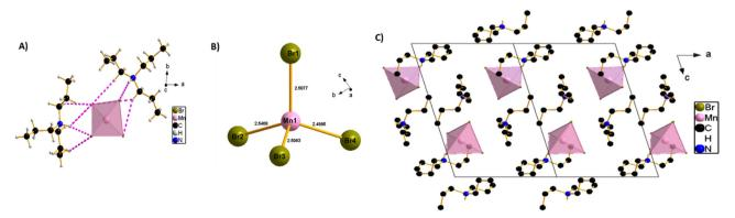
Scheme 1 (A) Crystal structure of  $(TPA)_2MnBr_4$  in the asymmetric part of the unit cell, the pink dashed line shows the H-bonds between tri-n-1propylammonium organic cations and  $[MnBr_4]^{2-}$  tetrahedral units. (B) Mn-Br distances in the single  $[MnBr_4]^{2-}$  tetrahedral units. (C) The packing diagram of (TPA)<sub>2</sub>MnBr<sub>4</sub> viewed from the b-direction at room temperature; all the H-atoms had been omitted for clarity.
